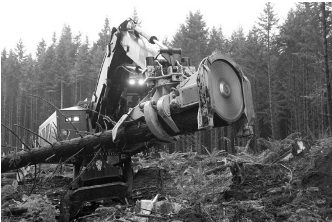
Figure 8 : Equipment used by Contestant One -- John Deere 959J Tracked Feller-Buncher (Source: Deere & Company Website)
