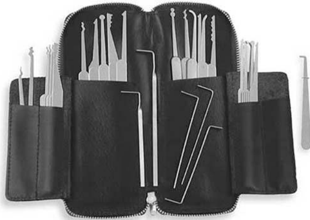
Figure 5.7 SouthOrd's 32 piece set contains everything you need to pick pin tumbler locks.
