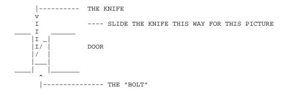
IF THE ROUND PART OF THE "BOLT" FACES YOU THEN WITH THE KNIFE, PUSH ON THE BOLT WITH THE BACK OF THE BLADE. AS YOU PUSH, SLIDE THE KNIFE TOWARDS THE SIDE OF THE DOOR. (SEE ILLUSTATION FOR CLARITY). YOU WILL SLOWLY MOVE IT. AND PRESTO! THE DOOR IS OPEN. THE TRICK IS TO SLIDE THE KNIFE AND PUSHING IT AT THE SAME TIME, AND HOLD ON TO THE DOOR KNOB. IF IT OPENS INWARDS, GET READY TO PUSH IT AS SOON AS THE KNIFE IS THRU THE "BOLT".
