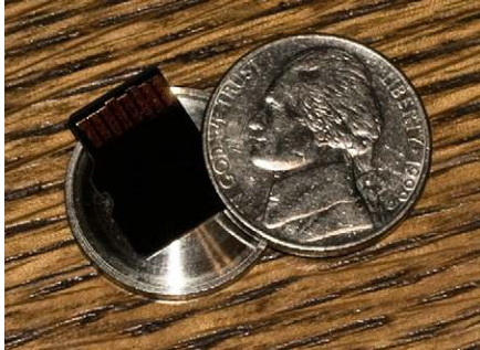
FIGURE 12.25 MiniSD Chip Concealed in Hollow Coin.
