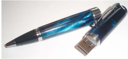
FIGURE 16.1 A Stealthy USB Storage Device.
