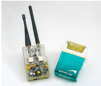
FIGURE 15.4 Wavebubble – A Self-Tuning, Wide-Bandwidth Portable RF Jammer. 13
