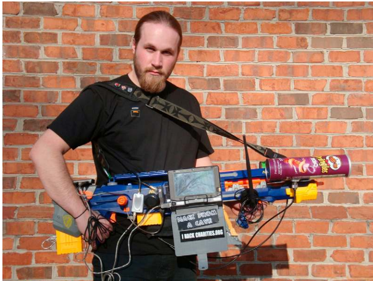
FIGURE 13.1 A Yagi Rifle.
