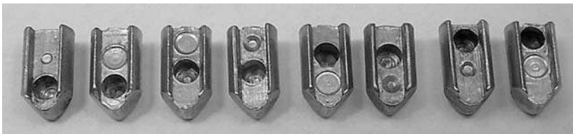
Figure 4.64: BiLock pins showing the four sizes and antipicking features.
