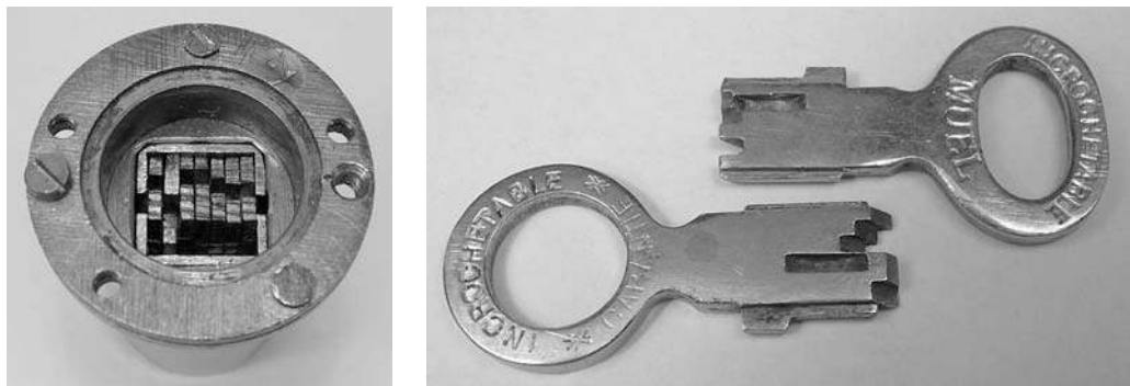
Figure 5.93: (Left) Rear of Muel 6-lever cylinder. (Right) Keys for 6-lever Muel locks.
