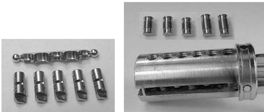
Figure 4.109: (Left) Left-handed finger pins and coded side-bar. (Right) Twin V-10 driver pins and plug with counter-millings on pin chambers.
