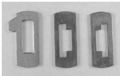
Figure 3.18: Conventional wafer-tumbler and two Bricard wafer-tumblers.
