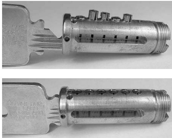
Figure 4.97: (Top) Medeco plug with key partially inserted. (Bottom) Key aligns pin slots with side-bar channel.
