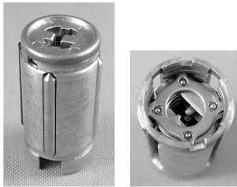
Figure 4.35: (Left) DOM Diamant shell with side-bars and frontal cap. (Right) View down keyway with cap removed.
