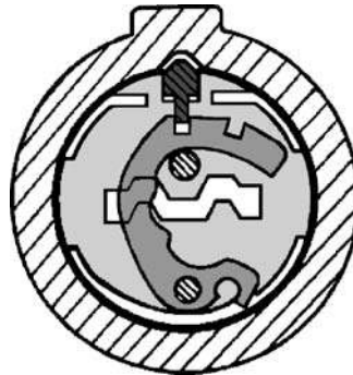
Figure 4.56: Design cross-section for the Miwa U9 lock (from N. Ikuo's 1999 patent JP 2000-291300).
