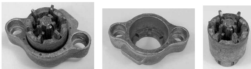
Figure 3.53: Supra 6-slider core and rear cap.
