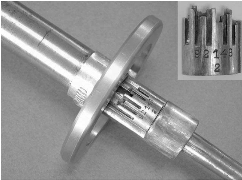
Figure 3.50: Plunger mechanism and escutcheon plate from Arnheim 14-slider axial safe lock with end-bitted stemless key loaded into the breech.
