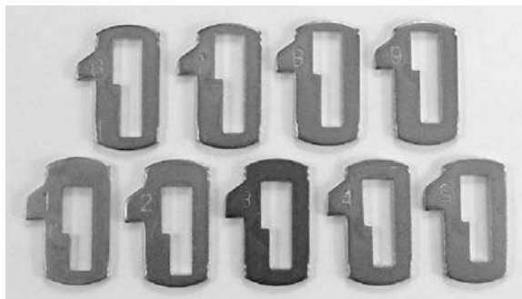
Figure 7.9: Set of wafers from Holden Commodore lock.
