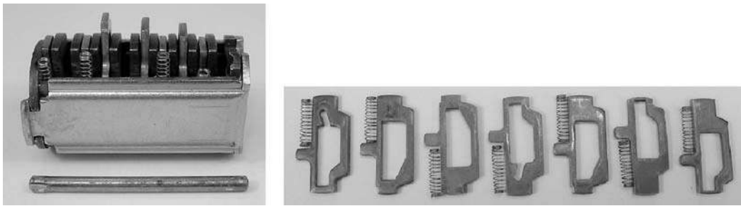
Figure 3.15: (Left) Miwa core and mounting rod with front cover removed. (Right) Set of wafers and springs.
