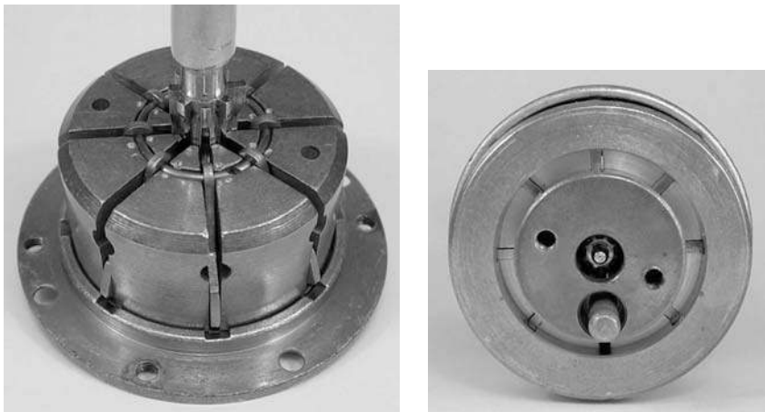
Figure 5.103: Operation of Monopole core: key aligns lever gates with gap at rear.
