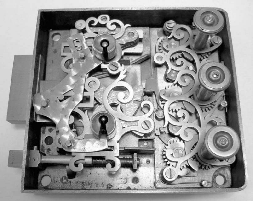
Figure 5.47: Triple-control Fichet safe deposit lock with 3-knob “click” mechanism. First, the three knobs must be set at the correct positions. The guard key is then inserted in the upper keyhole and turned to allow access for the renter’s key (top), which is inserted in the lower keyhole to operate the compound 5-lever lock. The fretting is ornamental—the original lock would have had a plain steel front plate.
