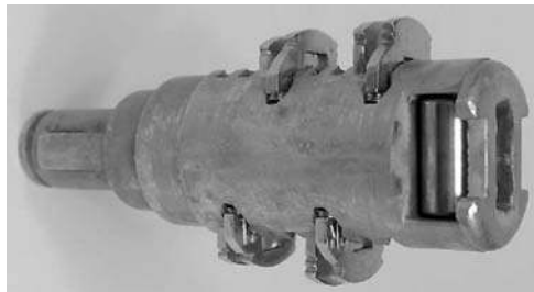
Figure 7.40: Volvo four-track plug.
