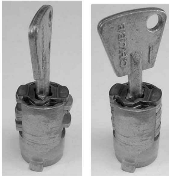
Figure 5.110: (Left) Chubb AVA core with key inserted. (Right) Key turned to align sliders with edge of shell.
