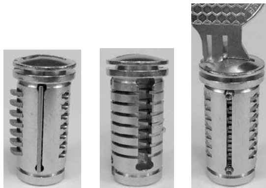
Figure 3.69: Views of Riella plug: rod side-bar in foreground (left); comb side-bar removed (middle); key aligns wafers with rod side-bar channel (right).
