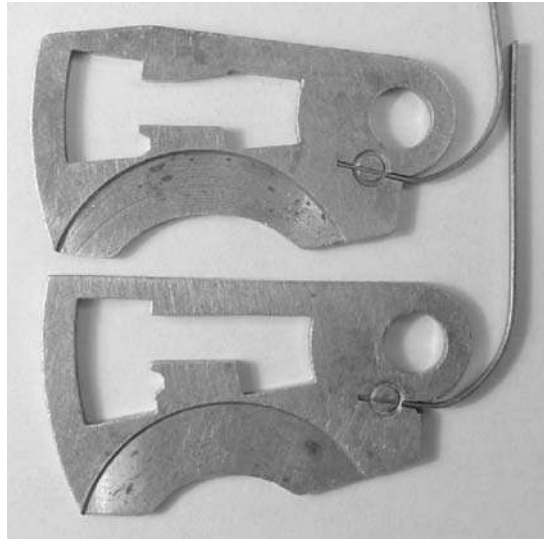
Figure 5.41: Levers from a Chubb 3G114 lock differ in respect of gate position and belly radius.
