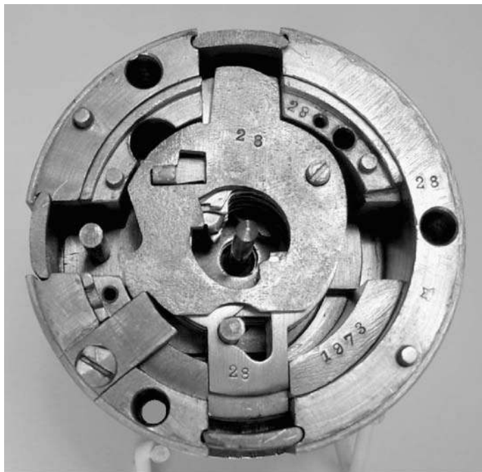
Figure 5.19: Panzer 12-lever lock from 1907 taking a 4-bitted key.
