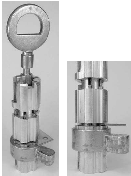
Figure 3.63: Vigie Picard core: key aligns slider gates with lower channel.
