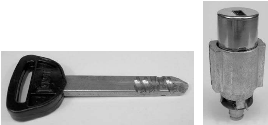
Figure 7.37: Lancia/Alpha-Romeo key and 10-pin lock barrel.
