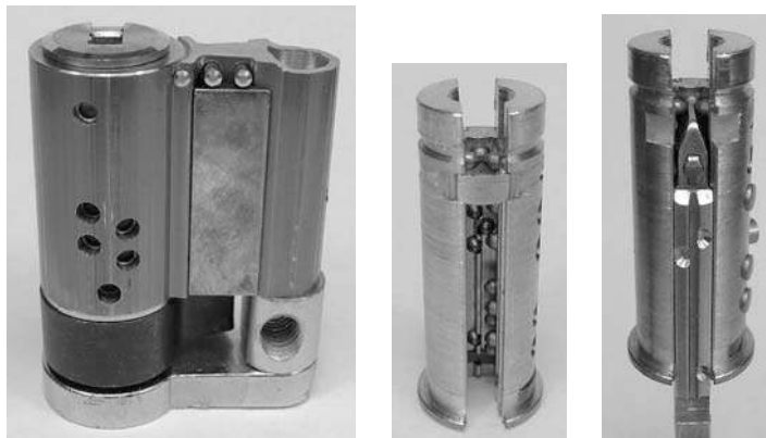
Figure 2.151: (Left) Radial NT cylinder with cover removed. (Center) View of plug with bridge for mobile. (Right) Key contacting check and blocking pins.
