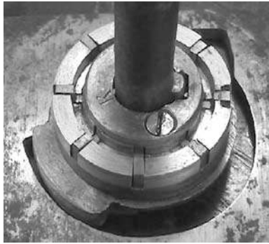
Figure 5.98: Key displaces levers to align gates with channel.
