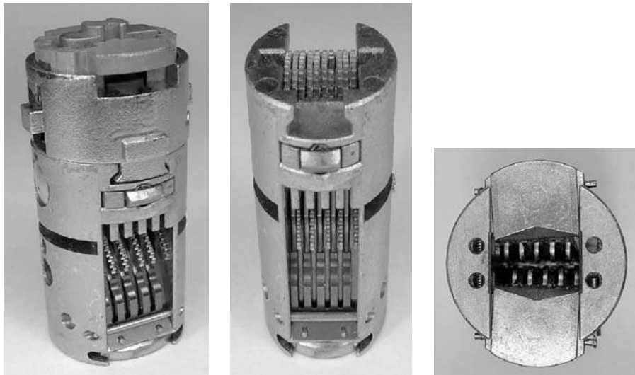
Figure 5.129: (Left) Fichet 787 core. (Middle) Core with rear section removed to show gears. (Right) View through gates at front of keyway.
