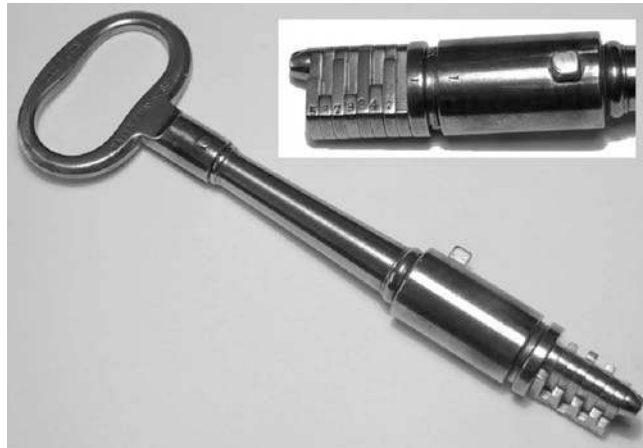
Figure 5.40: The key for Linus Yale Junior’s Magic Infallible bank lock had a removeable pod of 8 bits that could be rearranged by shuffling or flipping.
