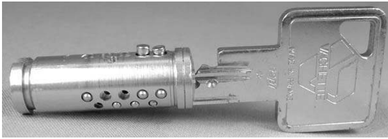
Figure 2.65: Vachette VIP plug with key partially inserted.
