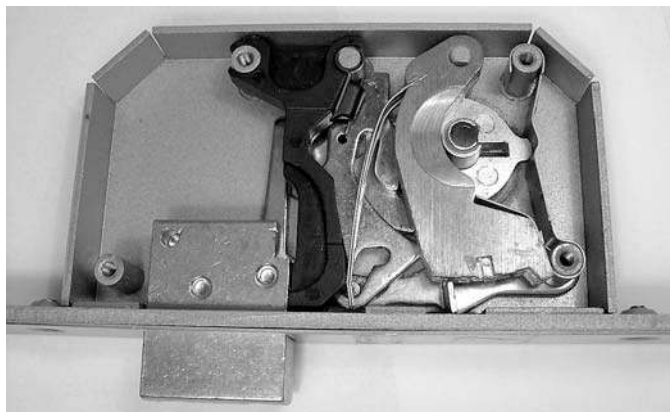
Figure 5.74: Chubb 3G110 mortice lock employing the Butter's system with cover on/off.
