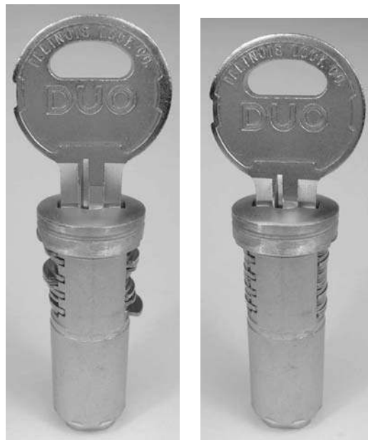
Figure 3.24: DUO plug with key partially and fully inserted.
