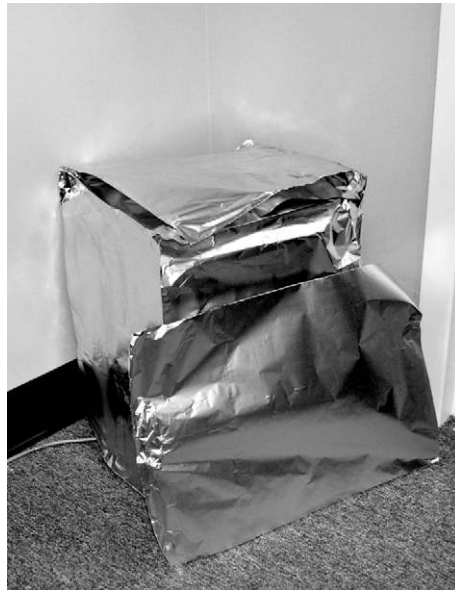
FIGURE 4.9 The tamper tests continue with aluminum foil covering the enclosure
