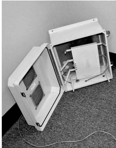
FIGURE 4.8 Standard enclosure and 802.11b/g/n access point used in our testing
