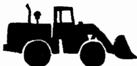
Articulated Loader (pivots in center)
