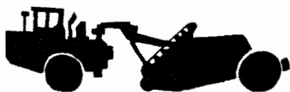
Scraper (w/2-wheeled tractor)
