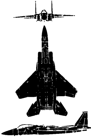
F-15 EAGLE (USA) WINGSPAN -- 13 METERS LENGTH ---- 19 METERS SPEED ----- 1,600 KNOTS RANGE ----- 3,200 KILOMETERS
