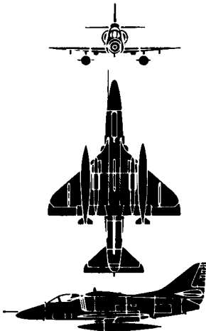
A-4 SKYHAWK (USA) WINGSPAN --- 8 METERS LENGTH ---- 12 METERS SPEED ----- 620 KNOTS RANGE ----- 3,307 KILOMETERS
