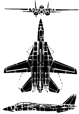
F-14 TOMCAT (USA) WINGSPAN -- 10/20 METERS LENGTH ---- 19 METERS SPEED ----- 1,500 KNOTS RANGE ----- 3,220 KILOMETERS
