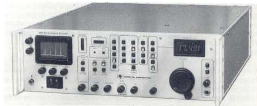
Figure 5.1. A superhet receiver. (Courtesy of Microtel Corp.)
