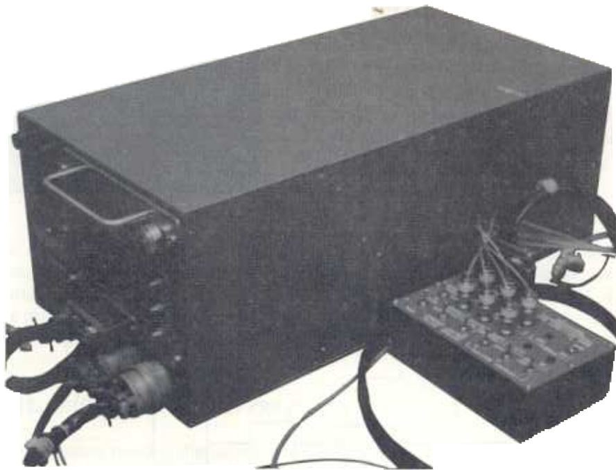
Figure 10.21. Digital microwave memory unit. (Fabricated by Whittaker Corp., courtesy of Avionics Laboratory, AFWAL.)
