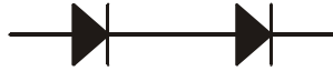
Figure 5.12 When the dominant failure mode of the diodes is shorting, connecting two diodes in series will ensure the circuit will continue to operate.
