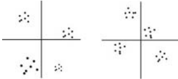
Figure 10.36 Two QAM or PSK constellations that exhibit different features that may be useful for modem identification.
