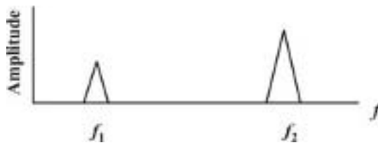
Figure 9.25 Signals at the input of a compressive receiver.
