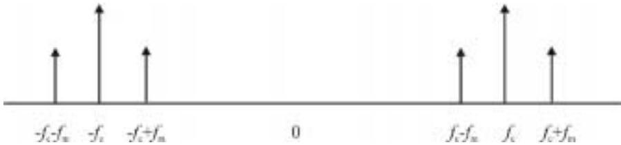
Figure 4.5 Amplitude spectrum of a signal that is AM-modulated with a tone.
