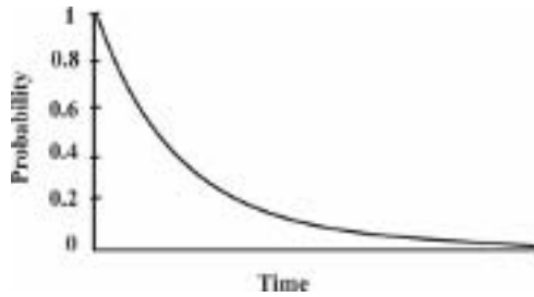
Figure 5.7 A typical reliability function.
