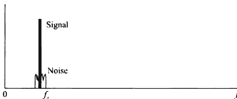
Figure 5.11 Spectrum of bandpass noise. In this case the bandpass filter limits the noise to only that necessary to pass the signal unfettered.
