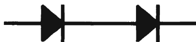
Figure C.12 When the dominant failure mode of the diodes is shorting, connecting two diodes in series will ensure the circuit will continue to operate.
