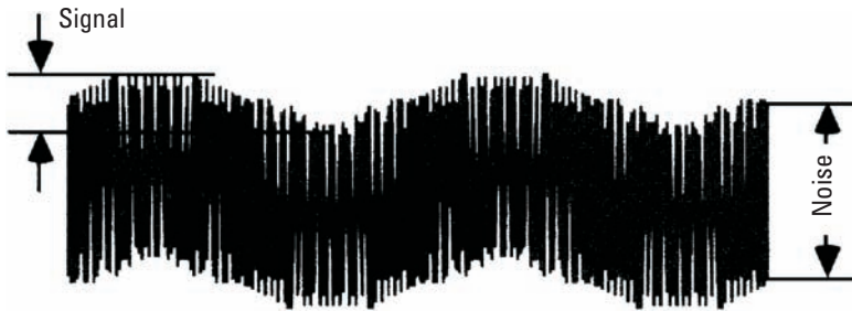
Figure 2.25 Low SNR signal with noise in time domain.
