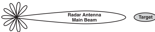
Figure 3.10 The peak gain point of the radar antenna either tracks the target or passes through its location during its scan.
