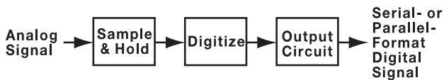
Figure 5.13 Digitization of an analog signal involves sampling, digitizing the amplitude of the sample, and formatting a serial or parallel digital signal.
