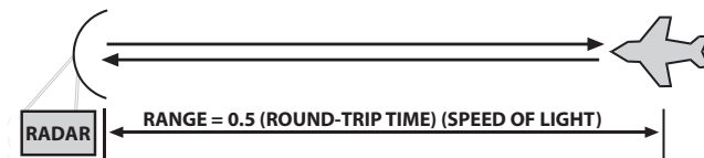
Figure 3.14 The radar measures the distance to a target as a function of the round-trip propagation time.
