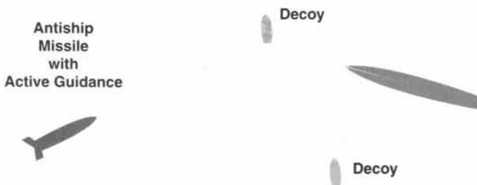
Figure 10.2 If a weapons sensor acquires a decoy before it detects a true target, it may attack the decoy, wasting an expensive guided missile.
