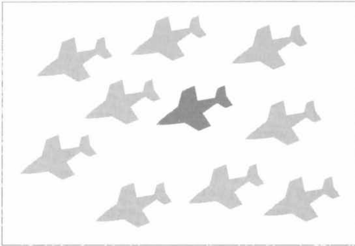
Figure 10.1 Saturation decoys force weapons sensors to deal with large numbers of apparent targets, reducing their ability to attack the real target.
