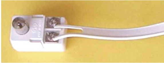
Figure 4.19 Balun. A 300 to 75-ohm balun, showing twin lead on the right-hand side.
