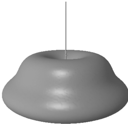
Figure 6.50 Helix normal mode 3D radiation pattern at f = 435 MHz.
