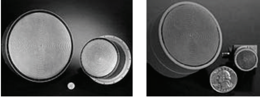
Figure 12.20 Cavity-backed spiral antennas. (Source: [11] © Cobham Sensor Systems. Reprinted with permission.)
