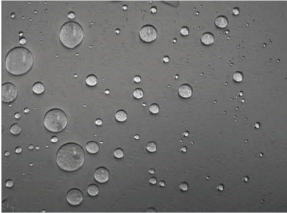
Figure 22.9 RF performance degradation is minimized with hydrophobic surfaces that cause water to bead. (Source: [1] © Microwave Product Digest 2008. Reprinted with permission.)
