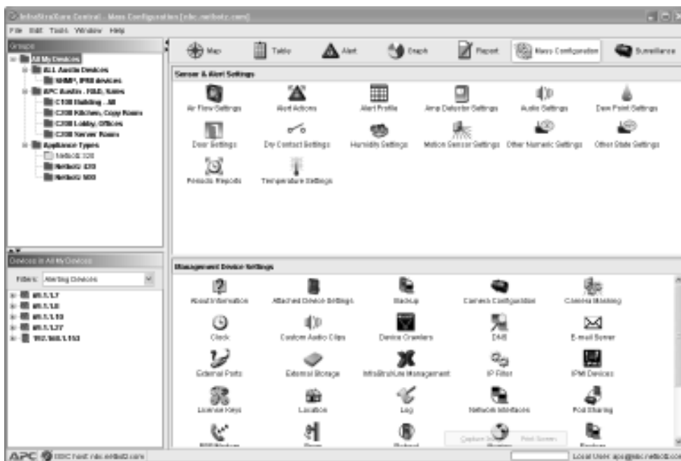
Figure 16.5 Console Connected to InfraStruXure Central While Performing Device Configuration (Source: APC/NetBotz)
