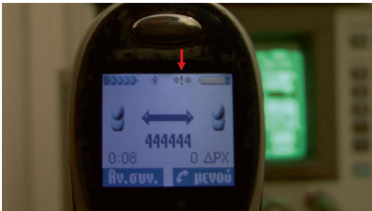
Fig. 5.22 The asterisks with the exclamation mark in the middle informs (those who are aware of their meaning) about the lack of encryption
