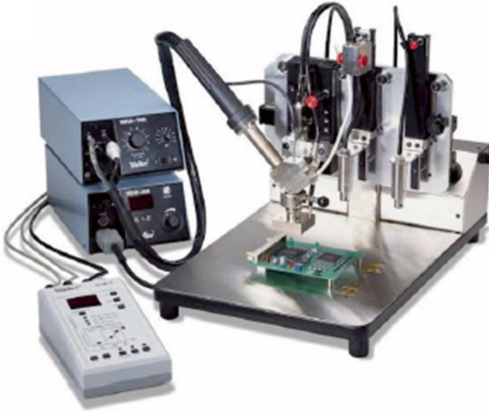
Fig. 5.7 Professional workstation for attaching/detaching electronic components
