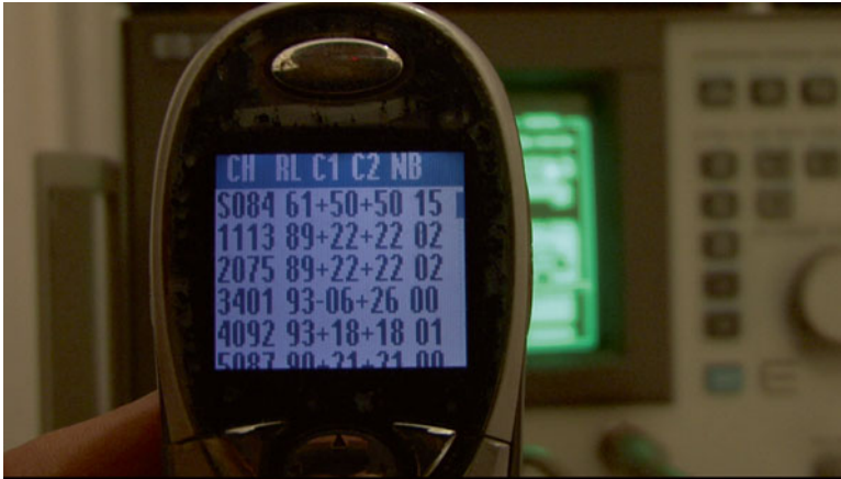
Fig. 5.17 Information about the available channels (ARFCN) and the received signal power as displayed using the Netmonitor software
