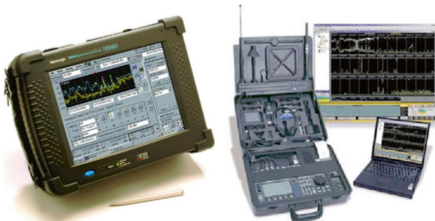
Fig. 7.6 Special spectrum analyzers-correlators for tapping detection
