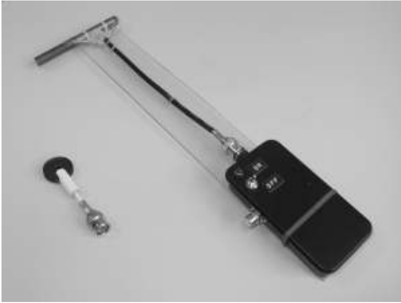
Fig. 10: VLF receiver with resonant ferrite coil. Due to the BNC connectors the coils can be changed easily. Lefthand a simple non-resonant pickup coil can be seen.
