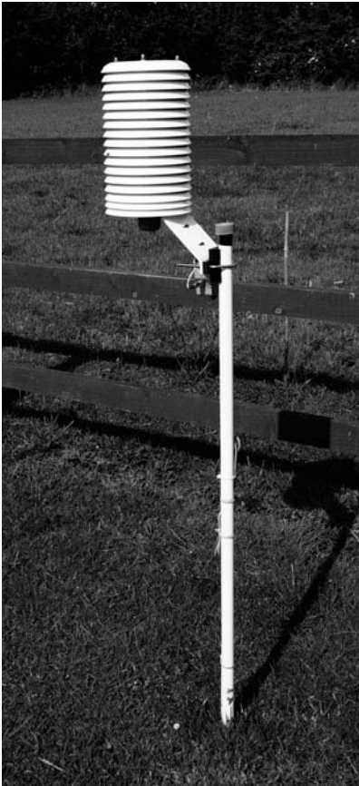
Figure 3.5. Tinytag Plus 2 TGP-4020 logger, here monitoring air temperatures inside a Campbell Scientific Met21 AWS screen. (Photograph by the author)
