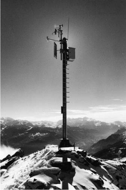
Figure 9.6. Automated snow, wind and weather AWS in the Swiss Alps, run by the Swiss Institute for Snow and Avalanche Research. The location is Vallée de la Sionne Windstation 'Crêta Besse' (4VDS1), in the Swiss Canton of Valais, at 2696 m above MSL. (Photograph courtesy of WSL-Institut für Schnee- und Lawinenforschung SLF, Davos, Switzerland)
