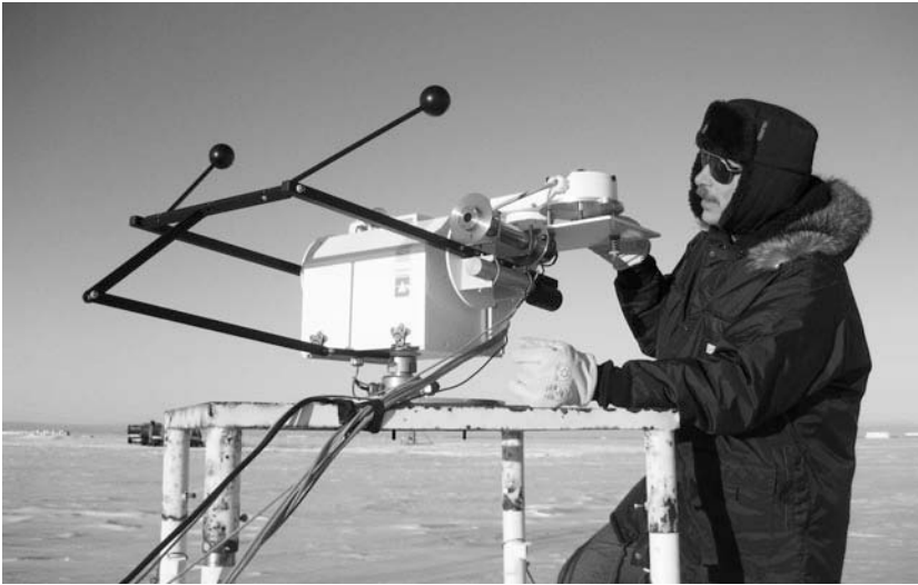
Figure 11.2. Solar radiation sensors at Neumayer station, Antarctica. The platform tracks the sun, and the two black spheres continuously shade one pyranometer measuring diffuse solar radiation and one pyrgeometer measuring long-wave downward radiation. One direct-incidence pyrhelometer (an Eppley Normal Incidence Pyrhelometer) is mounted above a four-quadrant sensor to the right of the platform in the photograph, directly above the observer's glove. (Photograph courtesy of Dr Gert König-Langlo of the World Radiation Monitoring Center at AWI)
