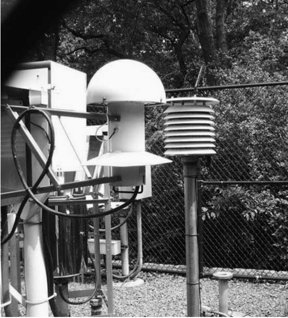
Figure 5.11. ASOS aspirated temperature shield (foreground) and MMTS (background) at New York's Central Park ASOS site, May 2010. (Photograph courtesy of Anthony Watts, www.surfacestations.org and Evan Jones)
