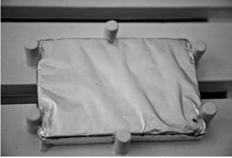
Figure 14.1. A simple hailgauge, constructed from a small sheet of aluminium foil stretched over a block of polystyrene and freely exposed to the weather. Dimensions are approximately 95 x 135 mm. (Photograph by the author)
