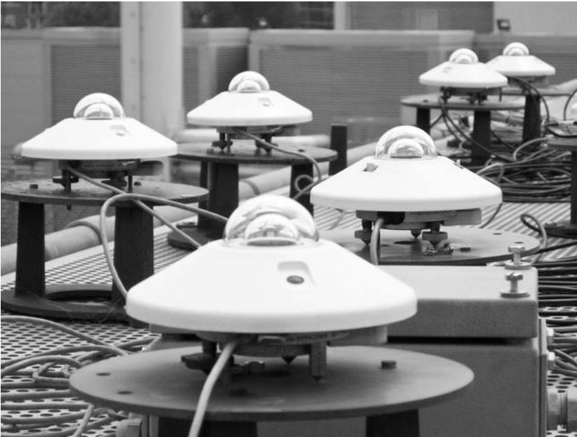
Figure 11.3. Banks of pyranometers at the UK Met Office test site in Exeter, England. (Photograph by the author)
