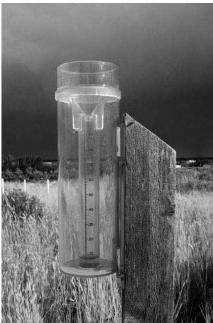
Figure 6.7. Four-inch plastic raingauge, as used in the U.S. CoCoRaHS network. (Photograph by Henry Reges, Colorado State University)
