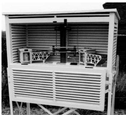
Figure 5.1. Large Stevenson screen from the UK showing the enclosed thermometers and two autographic recording instruments. The two vertically mounted units are the dry-bulb (left) and the wet-bulb; the horizontal thermometers are the maximum (top) and minimum. The two autographic paper-based instruments are a thermograph (left) and hygograph (right). Sandhurst, Berkshire, UK. (Photograph by the author)
