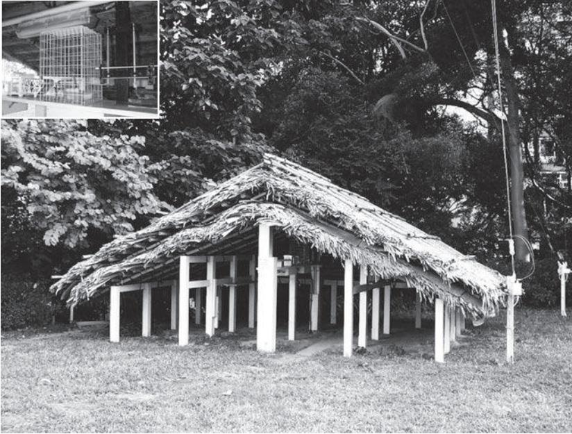
Figure 5.12. The thatched screen in the grounds of the Hong Kong Observatory, October 2001. Inset : screen interior. (Photographs by the author)
