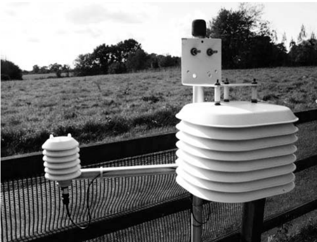
Figure 5.8. (Right of centre) Davis Instruments small plastic AWS screen, model 7714 (eight ‘stacked plates’, 18 × 18 cm, 14 cm high) shown alongside a smaller plastic AWS screen (left of centre – six ‘stacked plates’, 8 cm diameter, 9 cm high). Under comparative tests, the Davis unit performed well, but the smaller unit proved too small to provide adequate shielding against solar radiation and overheated badly in sunshine. (Photograph by the author)
