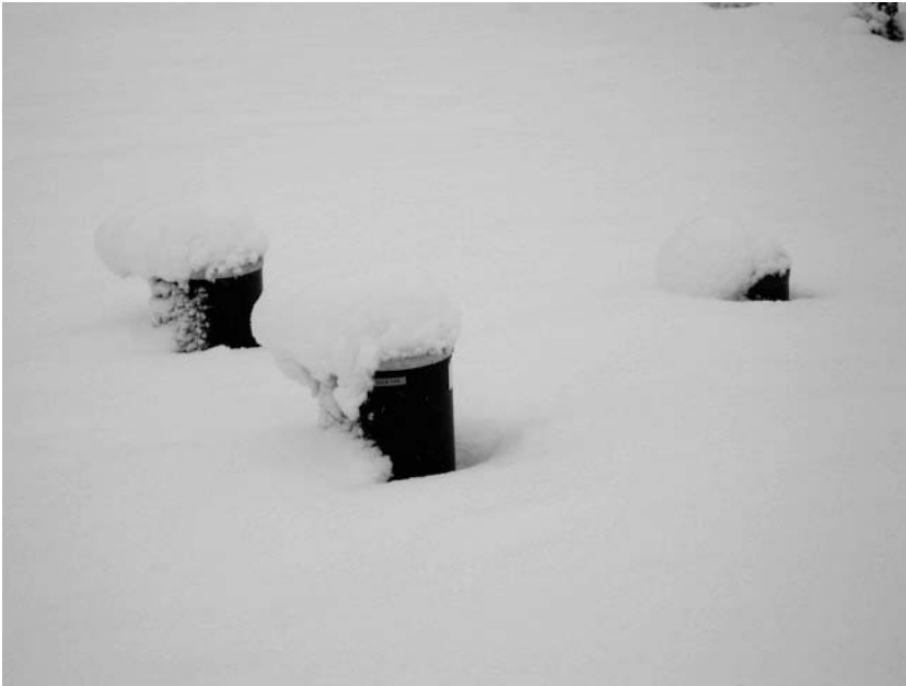
Figure 6.11. Manual and tipping-bucket raingauges gauges following heavy snowfall, January 2010. (Photograph by the author)
