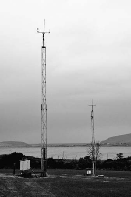
Figure 9.3. Anemometer and wind vane on 10 m masts in an exposed, open location; Valentia Observatory in south-west Ireland, October 2010. (Photograph by the author)
