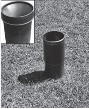
Figure 6.5. Standard UK rain gauge with rim at 30 cm above ground. See also Figure 6.8 . Inset: shallow-funnel rain gauge. These are liable to under-read in heavy rain, owing to outsplash, and are not recommended. (Photographs by the author)
