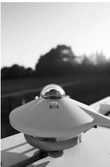
Figure 11.5. Kipp & Zonen CMP3 pyranometer. (Photograph by the author)
