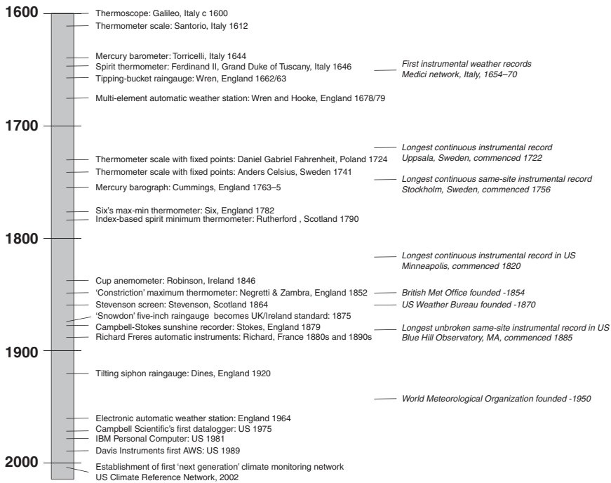
Figure 1.4. Four hundred year timeline showing key dates in the development of meteorological instruments and weather recording. For sources see references in the text.
