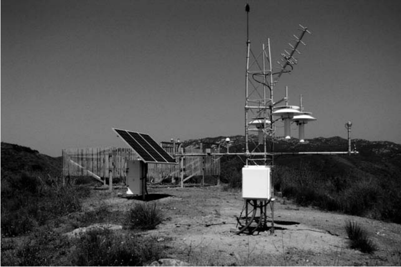
Figure 5.7. A site in the USCRN network (Santa Margarita Ecological Reserve, San Diego, California – 33.4°N, 117.2°W, 343 m / 1127 ft AMSL, 30 April 2008) showing the three aspirated screens which are used at over 100 sites across the United States to obtain parallel and fail-safe air temperature data. (Photograph courtesy of the National Oceanic and Atmospheric Administration/National Climate Data Center)
