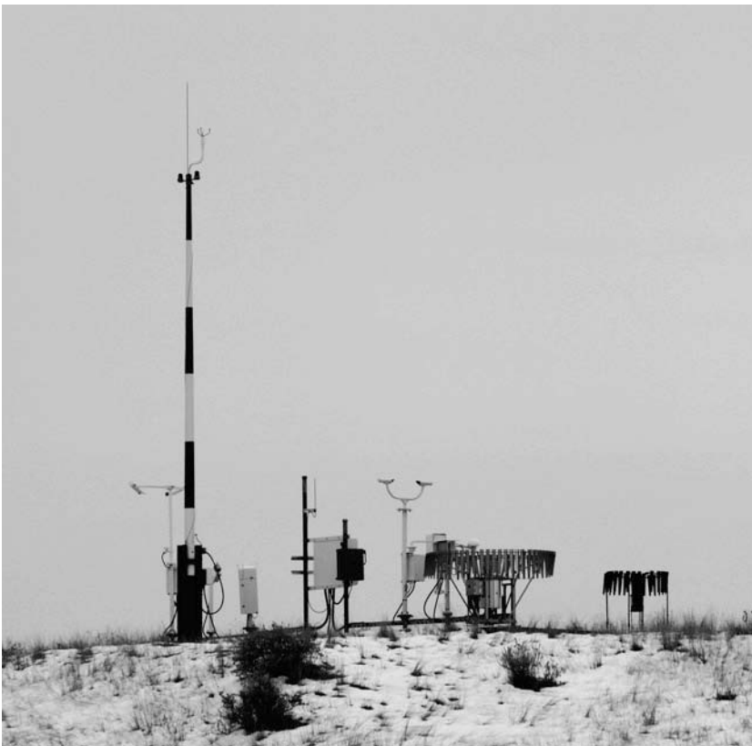
Figure 6.17. Alter wind shields (right of image) around ASOS raingauges at Cheyenne Airport, Wyoming 41.16°N, 104.81°W, 1876 m AMSL, October 2011. (Photograph by Henry Reges, Colorado State University)
