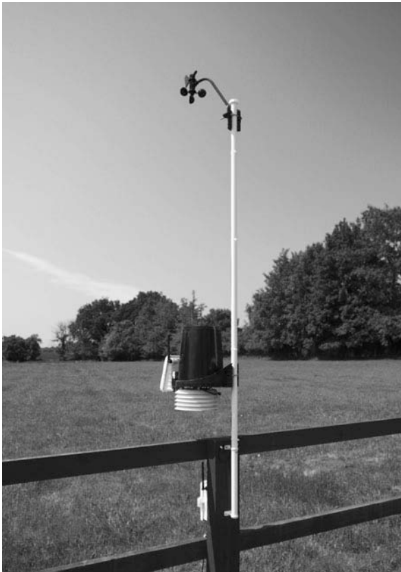
Figure 3.2. Exterior sensors of a Davis Instruments Vantage Pro2 AWS. (Photograph by the author)
