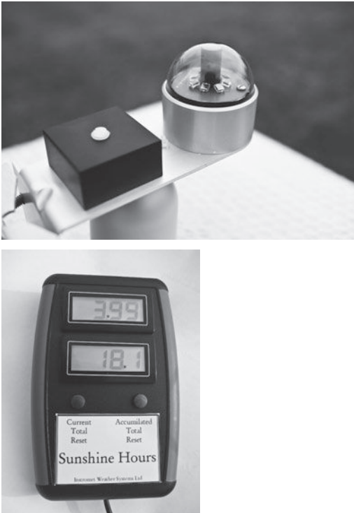
Figure 11.11. The Instromet electronic sunshine recorder. ( Top ) Sensor; ( bottom ) Display unit. Note the spelling of ‘Accumulated’! (Photographs by the author)
