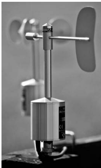
Figure 9.4. Vector Instruments cup anemometer, model A100, and wind vane, model W200P. (Photograph by the author)
