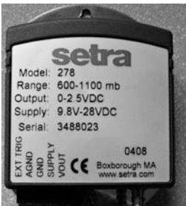
Figure 7.3. Modern electronic barometric pressure sensor; this unit is about 60 mm square. (Photograph by the author)
