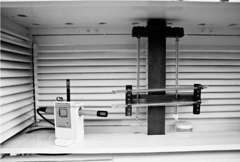
Figure 3.4. Tinytag TH-2500 logger (left of centre), here monitoring air temperatures inside a Stevenson screen alongside a platinum resistance sensor and conventional thermometry. (Photograph by the author)
