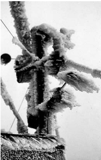
Figure 9.9. An early model automatic weather station on Cairn Gorm summit in Scotland (1245 m, 57°N, 3°W) in the 1980s, showing the problems of rime icing. (Photograph by Ian Strangeways)
