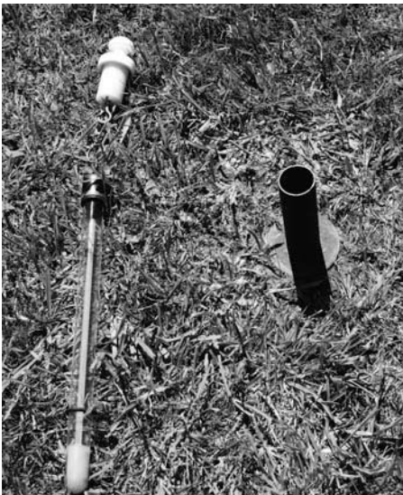
Figure 10.3. 30 cm depth earth thermometer (with wax-covered bulb), shown next to earth thermometer tube. (Photograph by the author)
