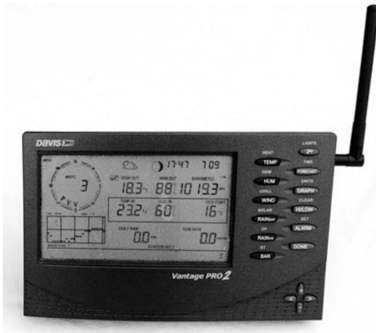
Figure 3.3. The interior display unit of a Davis Instruments Vantage Pro2 AWS. The logger fits into the back of this unit. (Photograph by the author)
