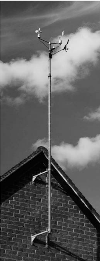
Figure 9.10. Anemometer, wind vane and Instromet sunshine recorder on mast attached to the gable end of a house; the anemometer is 11 m above ground level and 2.7 m above the apex of the roof-line. This photograph was taken from the south-west (the prevailing wind direction). (Photograph by the author)
