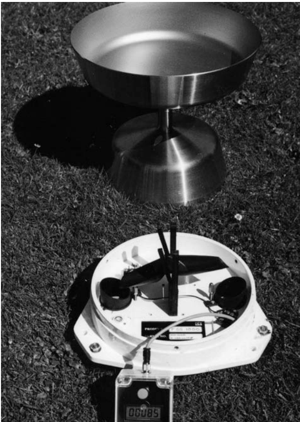
Figure 6.10. Tipping-bucket raingauge, showing details of the tipping-bucket mechanism. (Photograph by Ian Strangeways)
