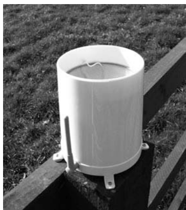
Figure 3.1. Entry-level wireless raingauge. (Photograph by the author)
