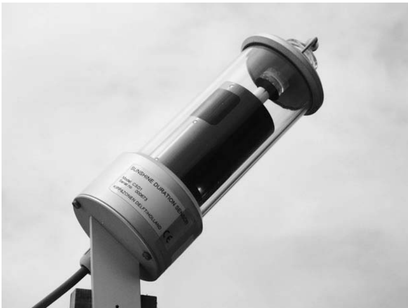
Figure 11.12. Kipp and Zonen CSD electronic sunshine recorder; UK Met Office, Exeter. (Photograph by the author)
