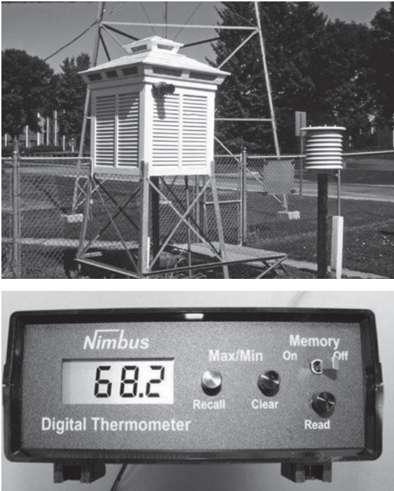
Figure 5.4. (Top) MMTS radiation shield (right of picture). The large shelter is a ‘Hazen’ louvred screen, fitted with an aspiration fan. Fort Collins, Colorado. (Photograph by Grant Goodge). (Bottom) MMTS interior display unit. (Photograph courtesy of National Weather Service)
