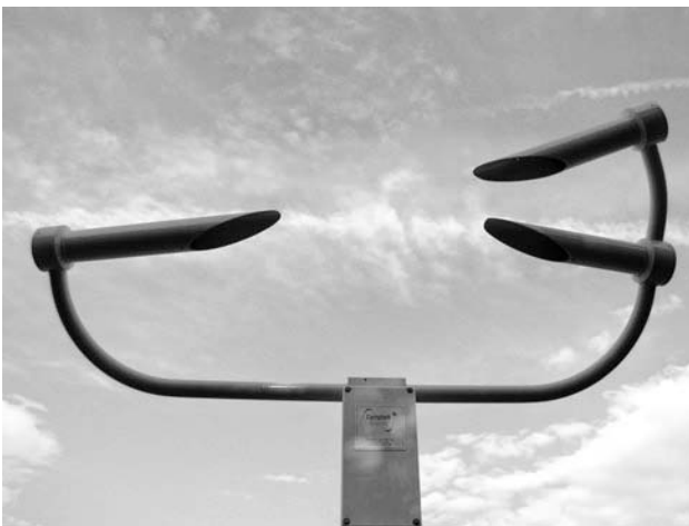
Figure 6.15. The Campbell Scientific PWS100 present weather sensor and optical rain gauge. (Photograph courtesy of Campbell Scientific)
