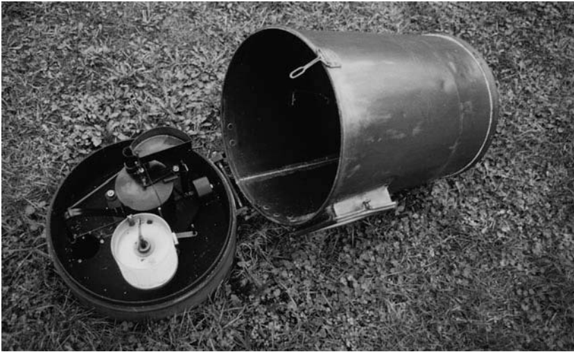
Figure 6.13. The Dines tilting siphon rain gauge (TSR). (Photograph by the author)
