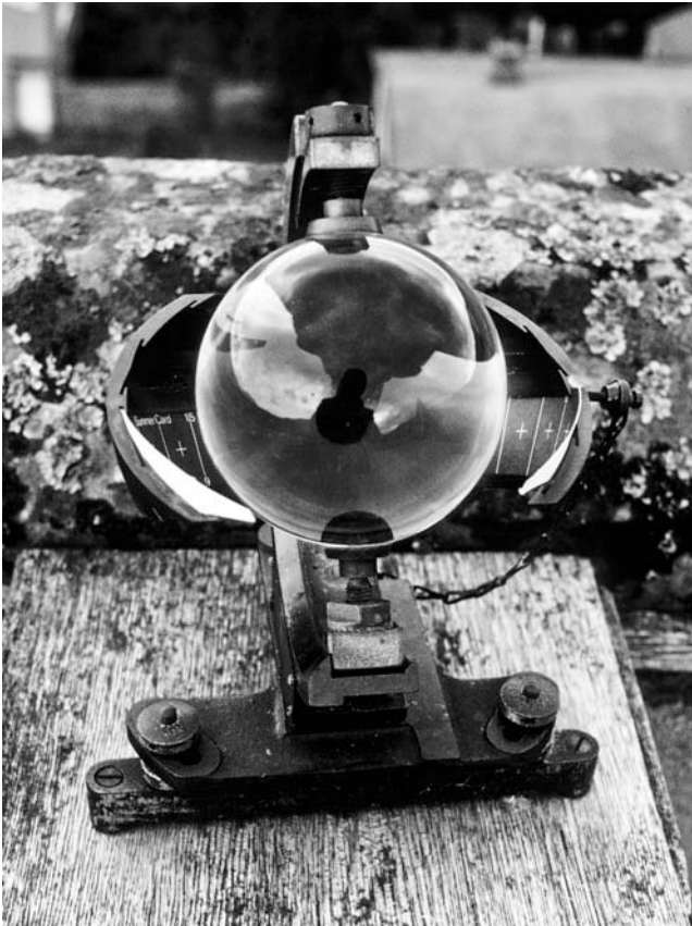
Figure 11.8. The Campbell-Stokes sunshine recorder at Braemar, Scotland. (Photograph by the author)
