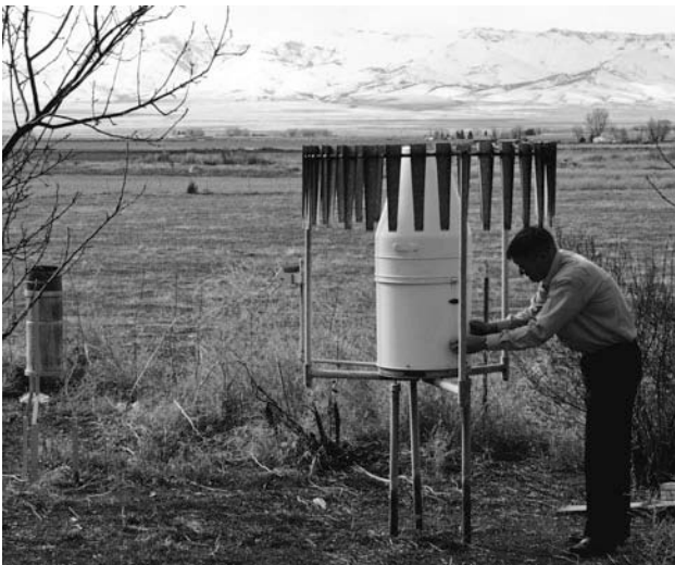
Figure 6.6. Standard U.S. National Weather Service rain gauges – standard manual eight-inch gauge (left), Fischer & Porter automatic gauge (right), being serviced by Gary Wicklund at Malta, Idaho, July 2010. (Photograph courtesy of Gary Wicklund and Vernon Preston)
