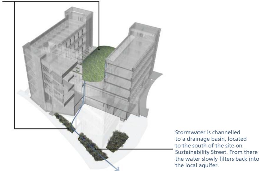
Figure 5.15 Rainwater to stormwater system. (Perkins+Will Architects)
