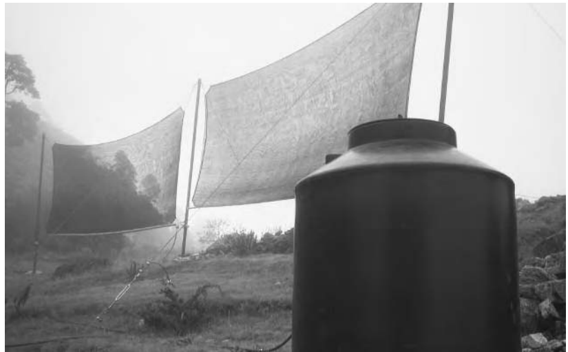
Fog collectors and tank in Guatemala
