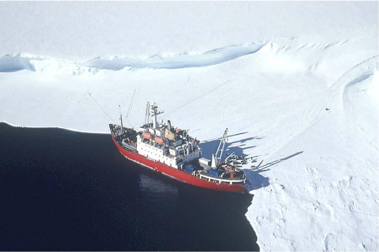
Iceport. The vessel is moored to fast ice in a creek in an ice shelf (Photograph 23)
