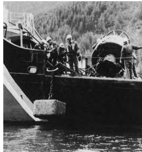
Figure 512. A sinker used to anchor a buoy.
