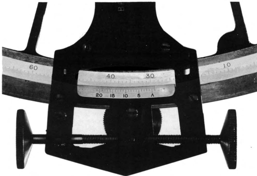
Figure 1608b. Vernier sextant set at 29^{\circ} 42' 30'' .
