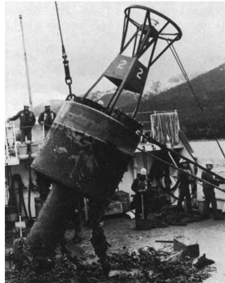
Figure 509. Buoy showing counterweight.
