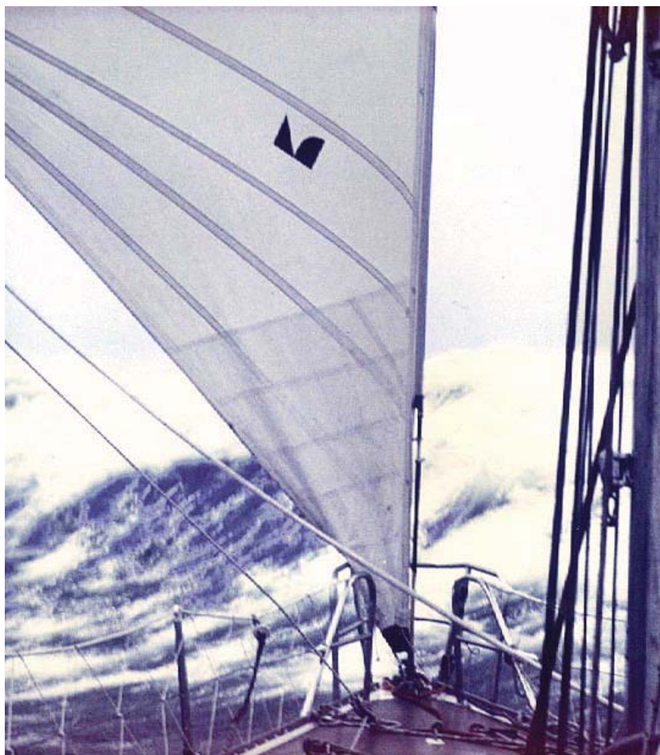
A high-clewed storm jib in the furious fifties aboard Ceramco New Zealand in the Whitbread Race. The clew is cut high so the sail will trim well off the wind as well as to windward. A high clew also keeps water out of the foot of the sail.
