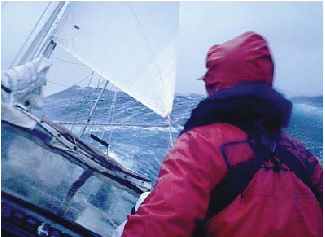
Sailing on a broad reach under trysail and storm jib. The trysail is a Hood radial panel sail rather than a cross-cut design. It is blowing in the 50-knot range, and seas are 20 to 30 feet (6 to 9m).
