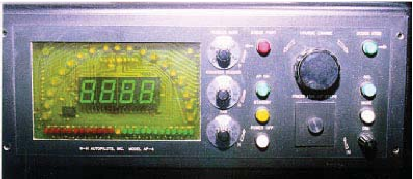
The WH autopilot control head on Beowulf is typical of what we've used on our clients' boats for over 15 years. Note the three manual controls for gain, counter rudder, and yaw (also known as dead band or sea state).
