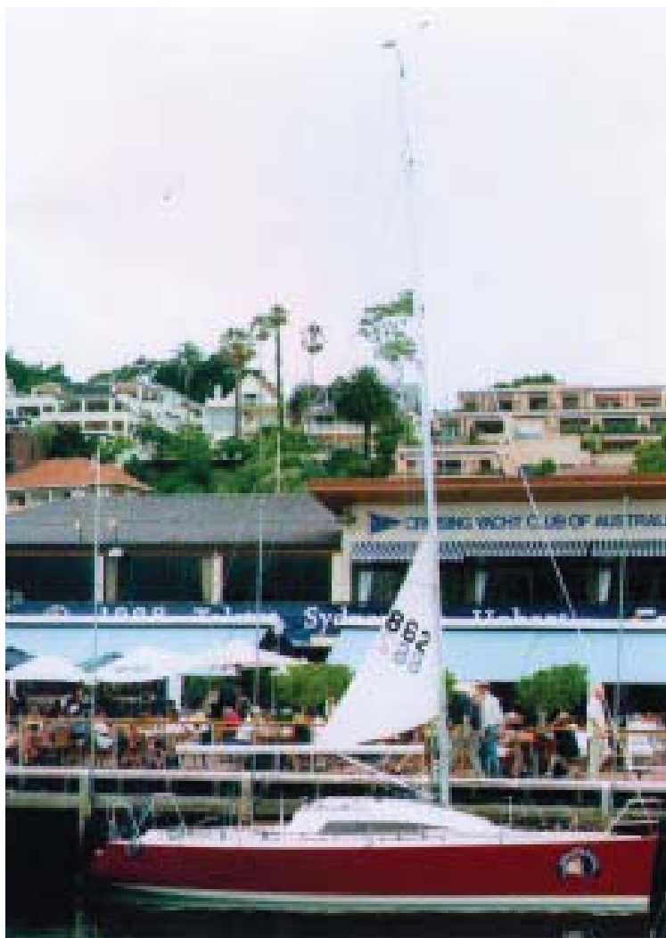
Bin Rouge wearing her trysail at the dock in front of the Cruising Yacht Club of Australia. This sail, from a smaller boat, measures just 10 feet (3m) on the luff, 8.5 feet (2.6m) on the foot, and 15 feet (4.3m) on the leech.
