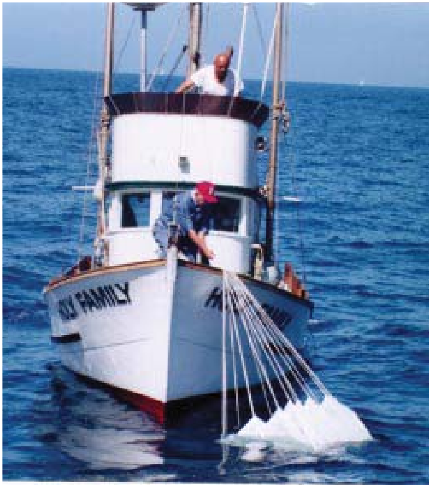
Commercial fishing boats were the first to use parachute anchors for heaving to when drifting at night or when waiting out bad weather.
