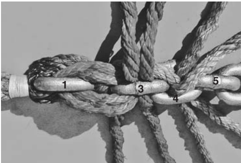
Square-line splice to chain, steps 3, 4, 5, and 6.
