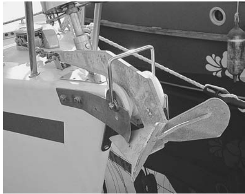
This bow-roller setup offers little lateral support. Thin flanges can be bent by just the rode, let alone chain or any other object it may contact.
