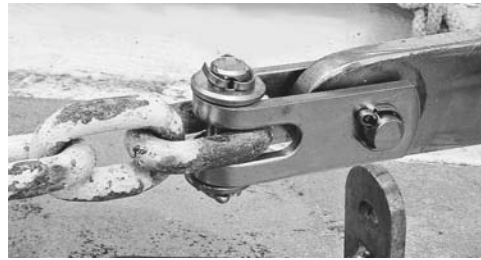
Attaching an anchor to chain with a toggle. This is the setup used on Alain's boat, SY Hylas .
