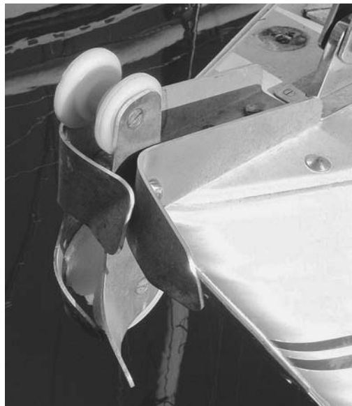
This is what happens if your flange plates are too thin; they buckle like an accordion.
