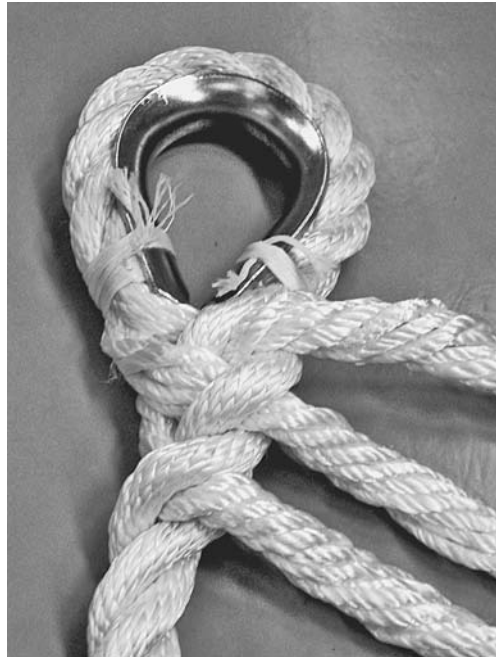
Splicing a thimble into anchor rode, step 7.
