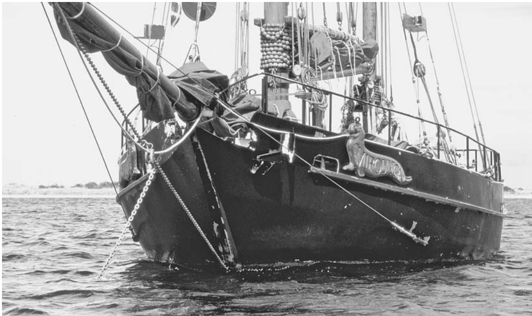
Bobstays are often problematic when anchoring, since the chain rode can grate against the stay, generating irritating noises.
