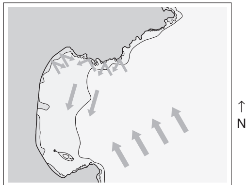
On this section of a retouched electronic chart, we've indicated that a skipper might want to take into account the backwash from wave action hitting the cliffs. Despite seemingly favorable conditions, the swell can be reflected at the rocky northern shoreline of the bay to create an uncomfortable chop in the entire anchorage.
