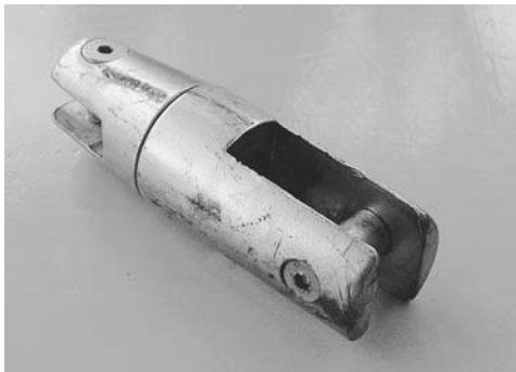
A chain-to-anchor connector with a swivel. Verify the authorized maximum load in linear and lateral directions.
