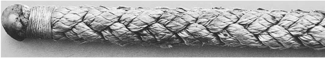
Especially comfortable to handle, eight-strand braided nylon is easily spliced to a chain leader.
