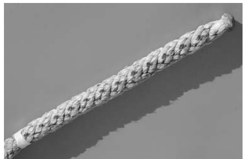
Square-line splice to chain, step 2. The twelfth turn is marked with whipping.
