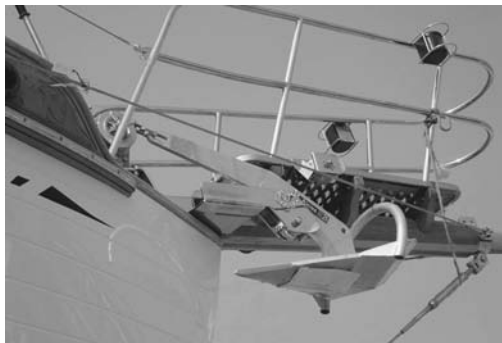
One solution to having an anchor at the bowsprit is to place the bow roller on one side or the other of the bowsprit.
