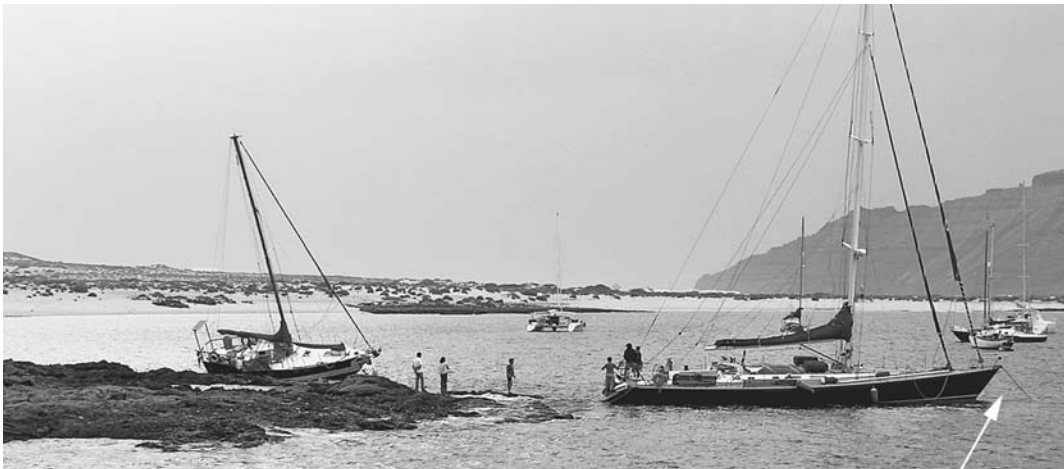
Off La Graciosa in the northern Canary Islands, the anchors of these two boats slipped and did not reset, with the result that both yachts drifted onto the rocks.
