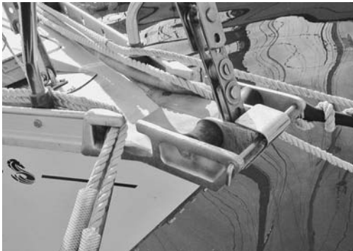
Production boats often have undersized bow rollers. It is doubtful that this roller can accommodate the shaft of most new-generation anchors. The smooth black plastic roller has a very small diameter and no groove in the center to guide the chain leader.
