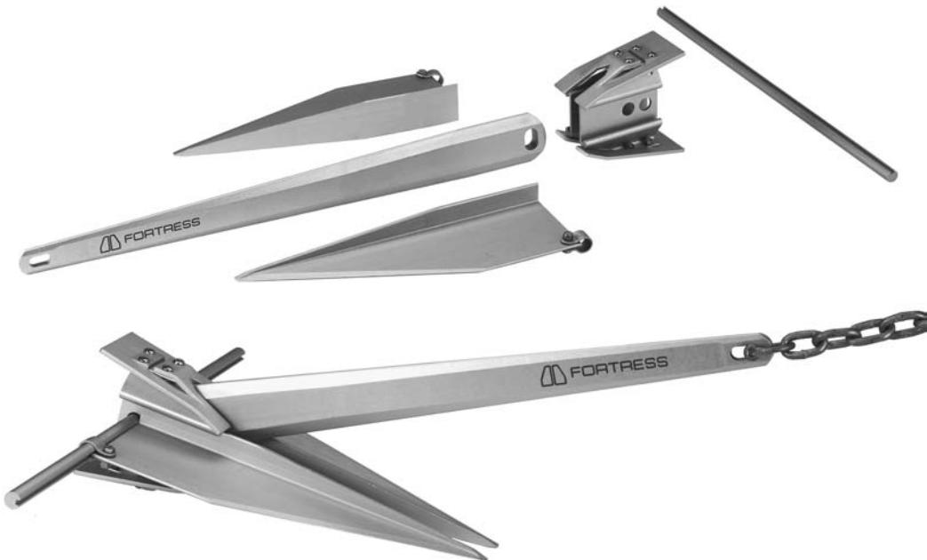
Fortress anchor. In its disassembled form, make sure to keep all five parts together! The angle of the fluke is adjustable from 32° to 45°.
