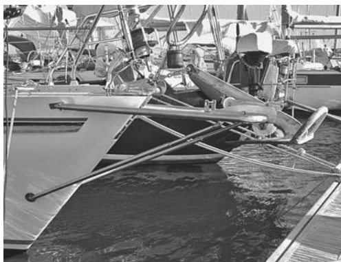
A bow platform with a heavy roll-bar anchor exacerbates pitching of the vessel in high seas.
