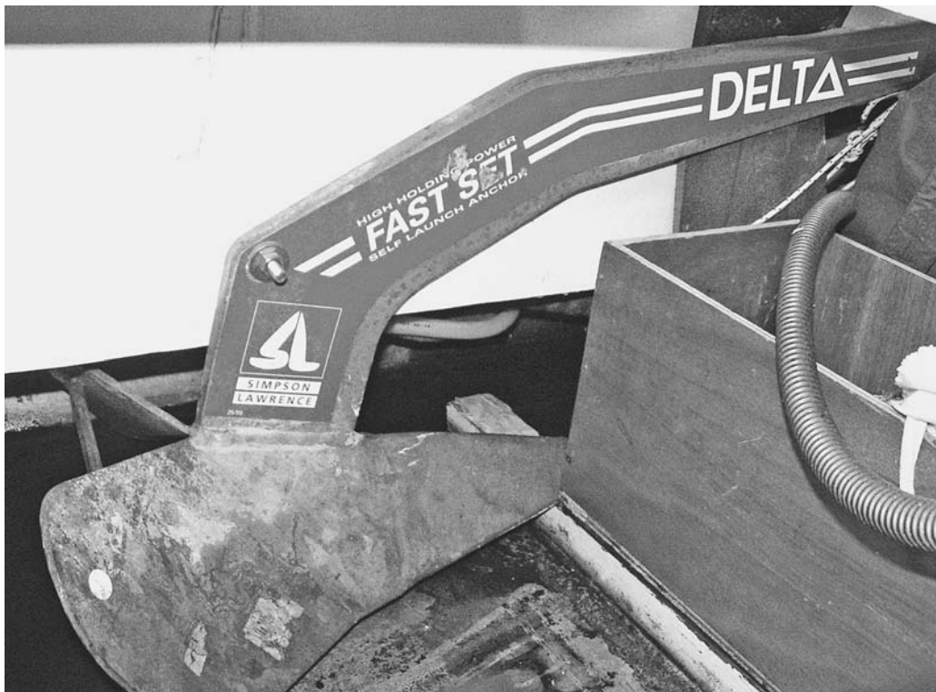
A spare anchor for emergency purposes can come in handy for offshore cruising sailboats. To keep the weight as close to the center of gravity as possible, the spare anchor should be securely fastened with a bolt, nut, and washer to a bulkhead, like this Delta anchor.
