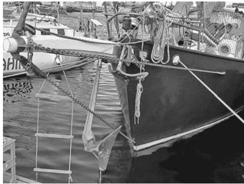
This chain bobstay obstructs both anchors. Two full-chain rodes will probably cause sleepless nights due to the chain-on-chain grinding noise.
