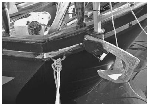
A stern anchor mount. The lateral white nylon wheels on the sides prevent line chafe.
