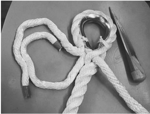
Splicing a thimble into anchor rode, step 5.
