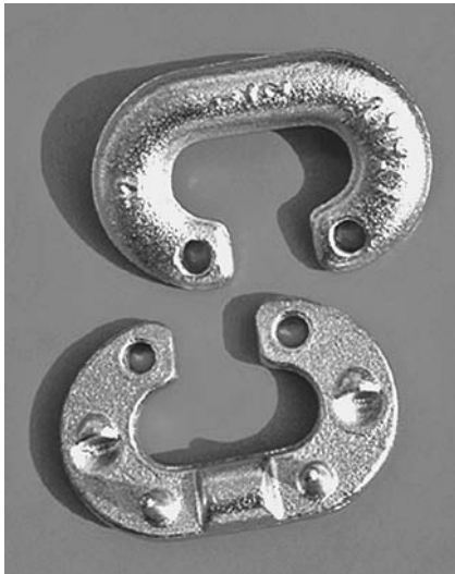
This riveted chain link is split laterally, significantly reducing its breaking strength.
