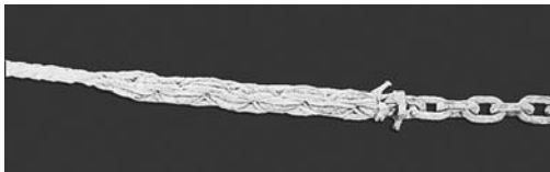
Chain-nylon chain splice.
