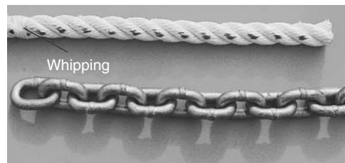
Three-strand splice to chain, steps 1 and 2.
