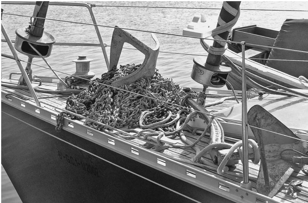
The yacht on the right in the photo on page 11 was riding on this full-chain rode during the storm. Note the bent shaft of the CQR anchor on the right.
