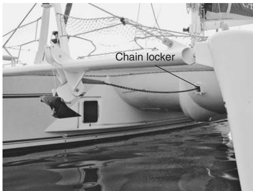
A catamaran's chain locker, located close to the mast foot, close to the boat's center of gravity. (Courtesy Catana Catamarans)
