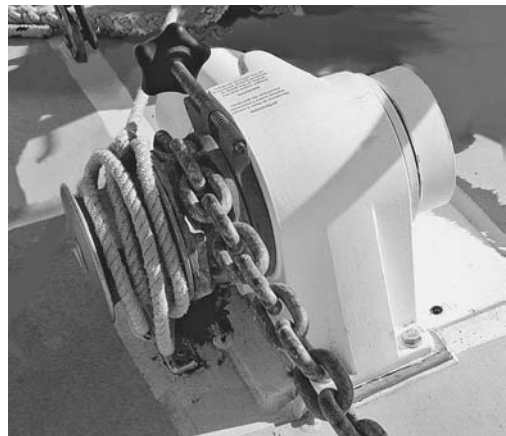
Horizontal windlass with chain-only gypsy and a separate warping drum. Beware! Keep your hands safe during the tricky shifting maneuver from the chain leader to the rode's line section.
