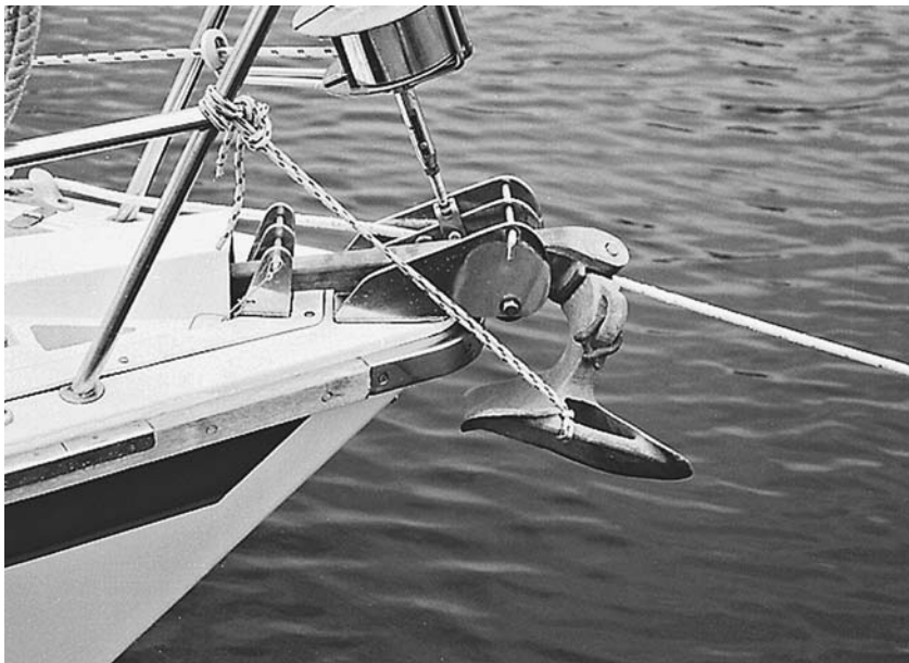
Neither of these two safety bolt systems actually prevent the anchors from unintentional launch. Note how the skipper needed to secure the crown of the articulating CQR to prevent it from flopping around.
