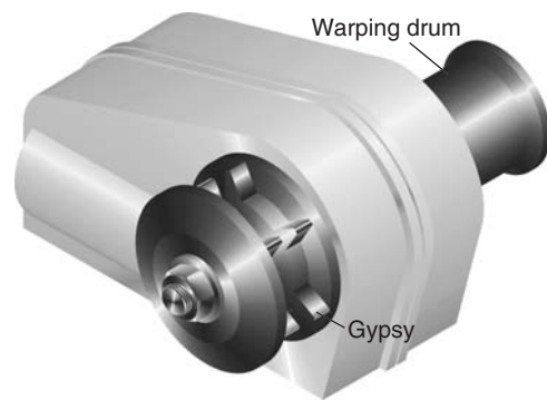
Horizontal windlass with horizontal motor shaft perpendicular to the chain gypsy.
