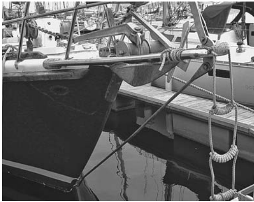
The bobstay of this bowsprit might cause serious damage to an anchor line. See our solution with a snubber and chain hook attached at the bobstay chainplate.
