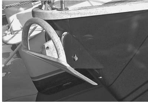
A custom-fitted bow roller for a roll-bar anchor with large, rounded flanges.
