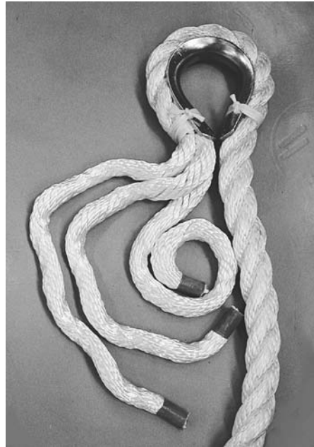
Splicing a thimble into anchor rode, steps 1 through 4.
