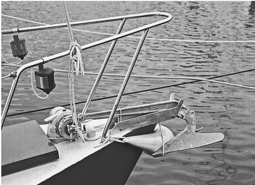
This crescent-shaped bow fender helps avoid hull damage.
