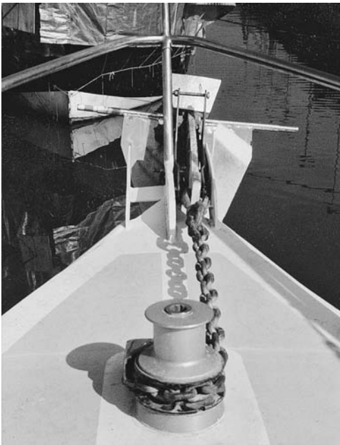
Vertical windlass with combined rope-chain gypsy and warping drum.
