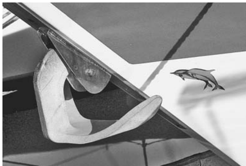
A custom-built bow roller is fine, but it may only accommodate one type of anchor. This bow roller is integrated in the hull to fit a claw anchor.
