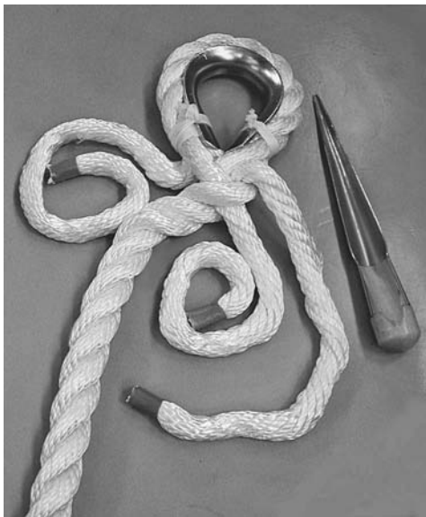
Splicing a thimble into anchor rode, step 6.
