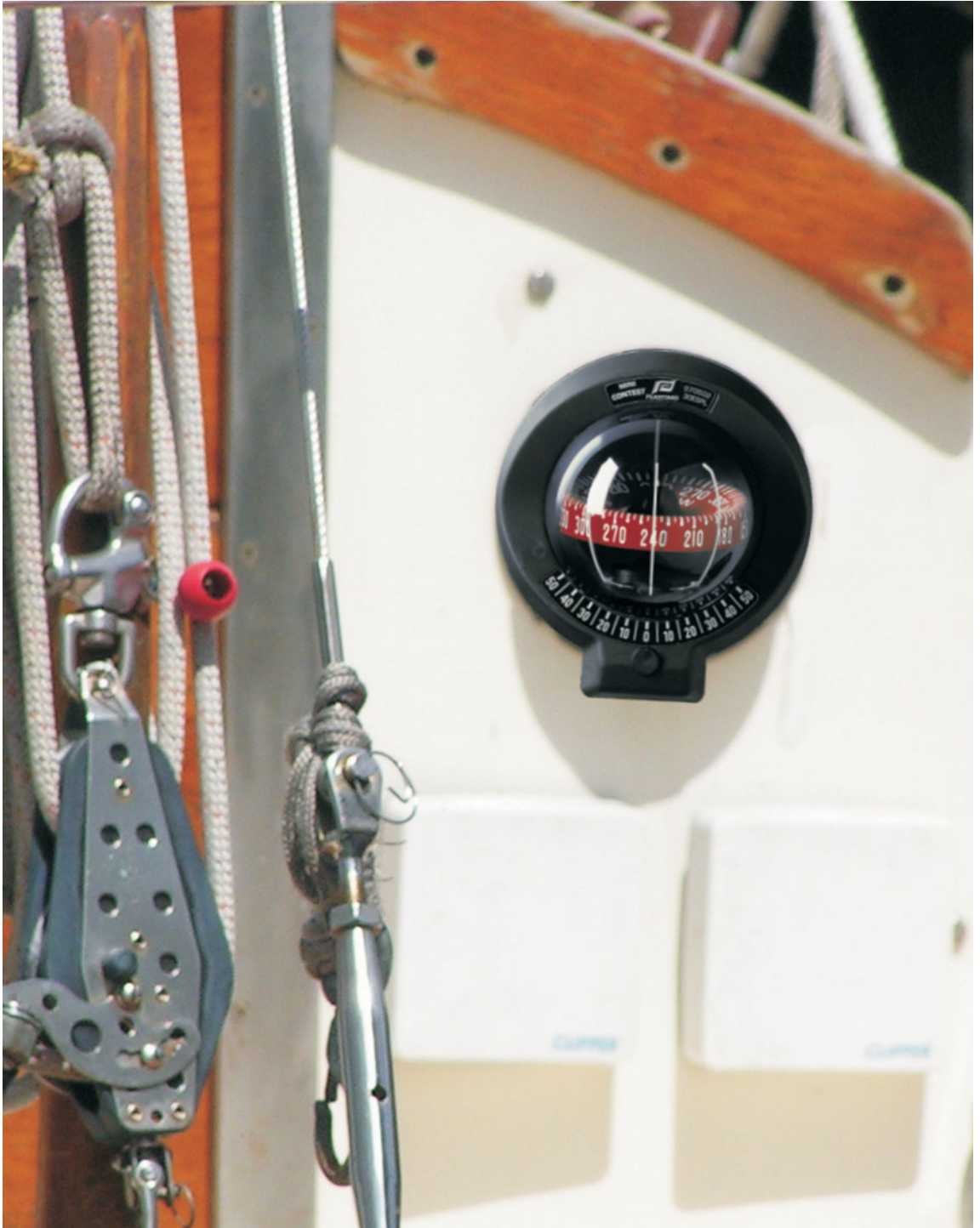
Fig 13a A bulkhead-mounted steering compass on a sailing cruiser.
