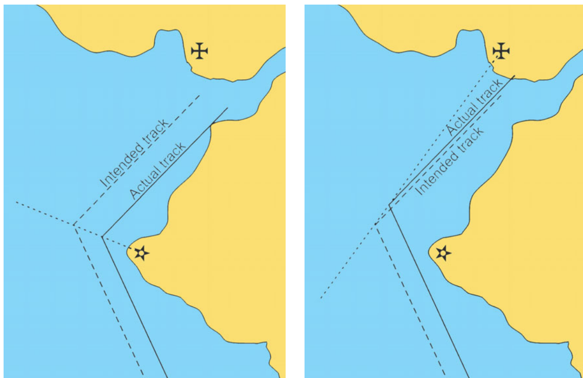
Fig 120 When using a compass bearing to decide when to alter course, it is better to use a landmark which will be directly ahead or astern on the new course than one which is abeam.
