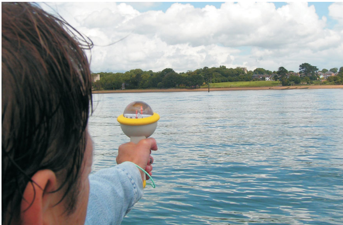
Fig 14 A hand-bearing compass. On this type, the fore sight and back sight are inside the compass bowl.
