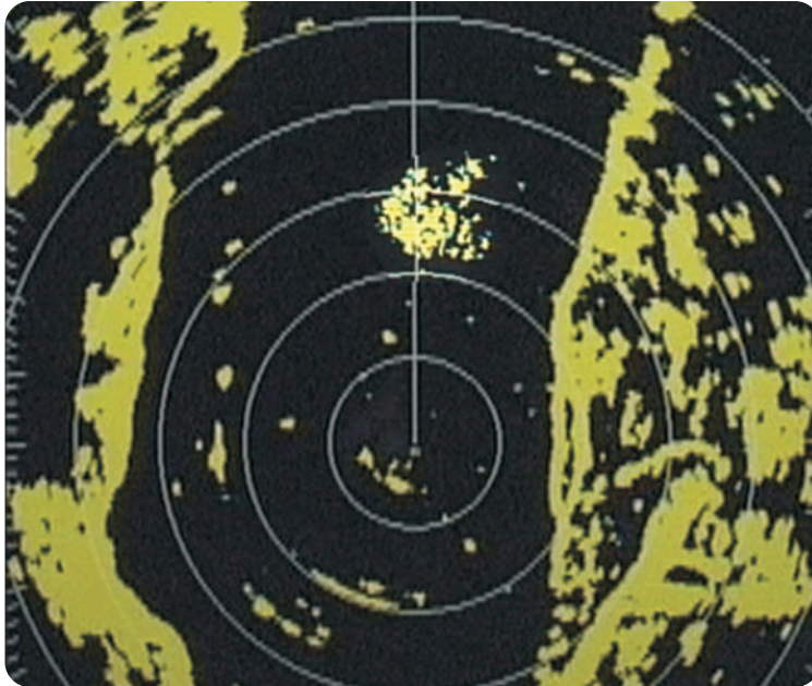
Fig 93 Rain clutter (the speckled patch just above the centre of this radar picture) can obscure contacts.
