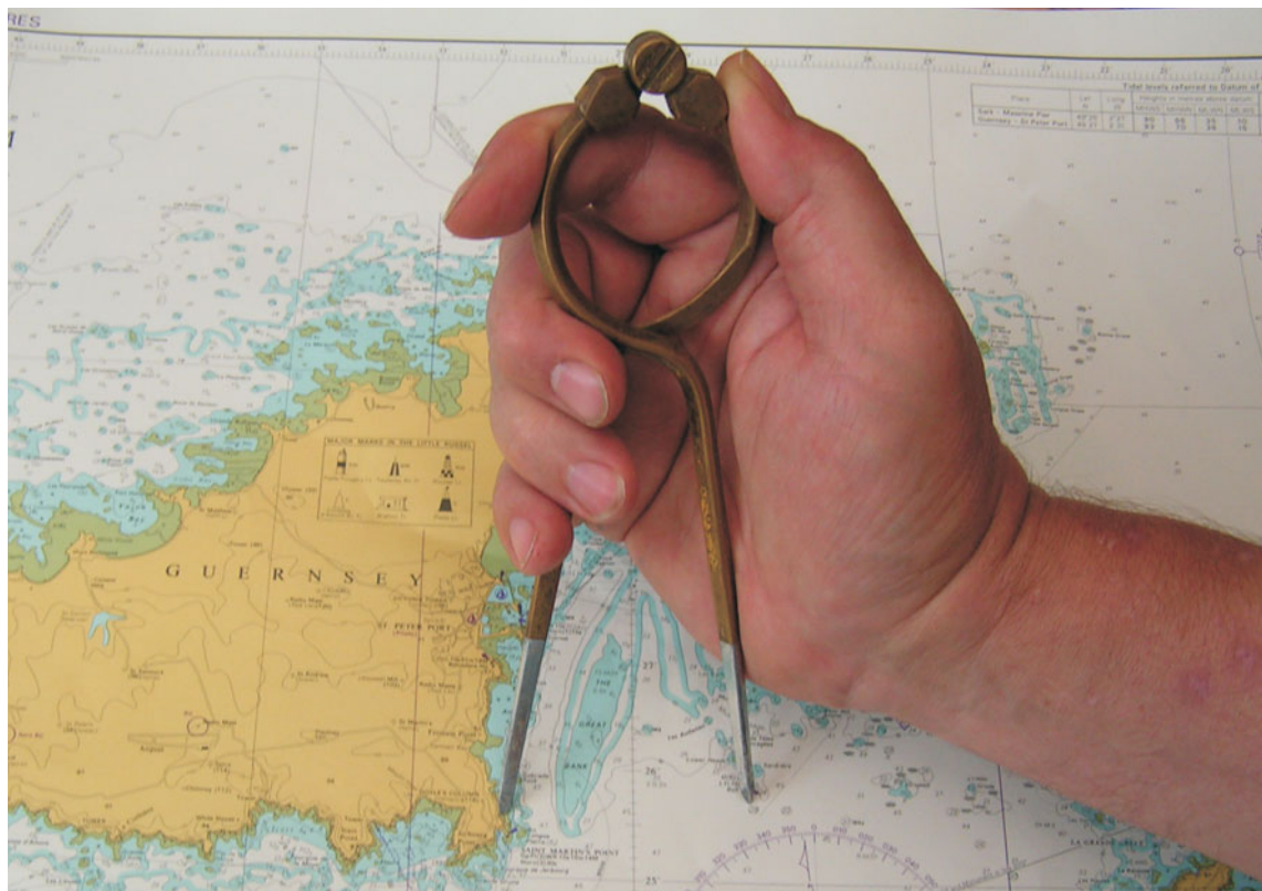
Fig 12 Bow dividers, which can be used with one hand, are ideal for measuring distances on a chart.
