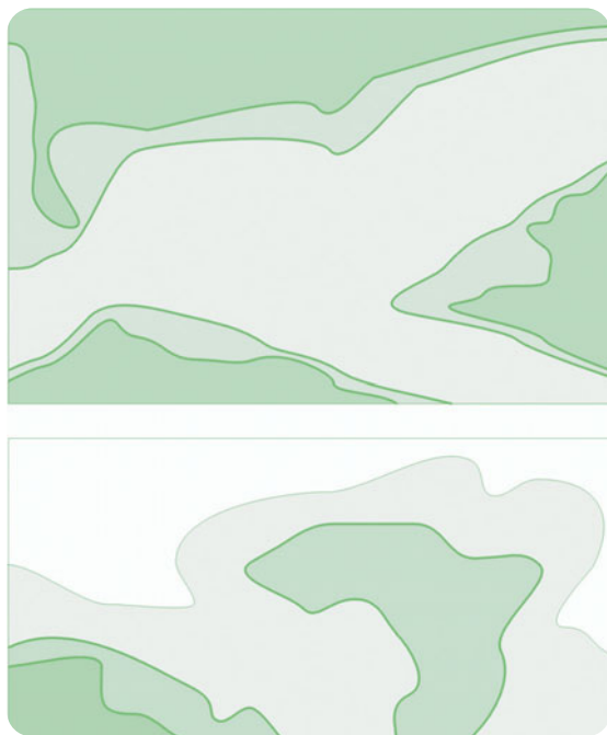
Fig 113 An echo sounder can be used to follow depth contours, but beware of forked channels (top) and hooked contours (bottom).
