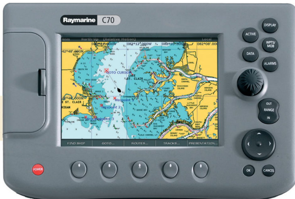
Fig 27a As the price of computing power and displays has fallen, chart plotters such as this Raymarine C70 have largely taken over from stand-alone GPS receivers.
