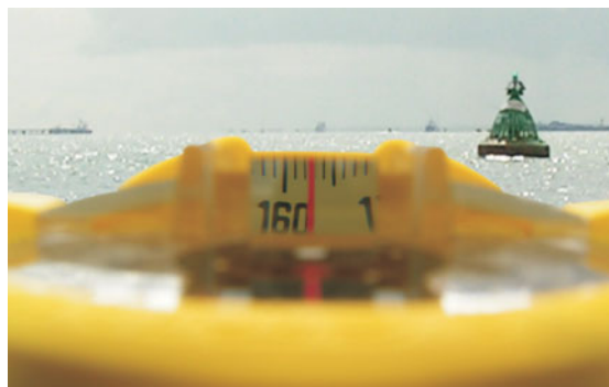
Fig 122 When using a back bearing, it is usually easier to sight along the correct bearing to see whether the mark is to the left or the right than to take a bearing of the mark and try to figure out the implications.
