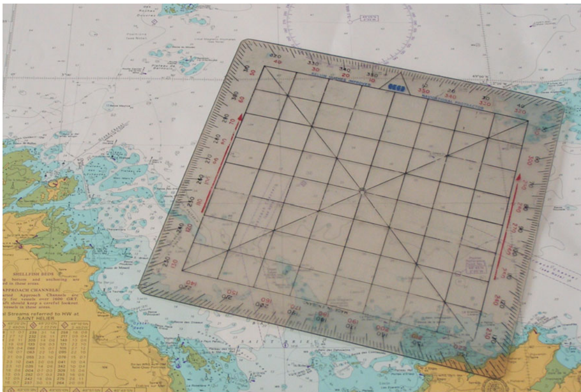
Fig 21 A Kelvin Hughes protractor – a larger and thicker variant of the Douglas protractor.
