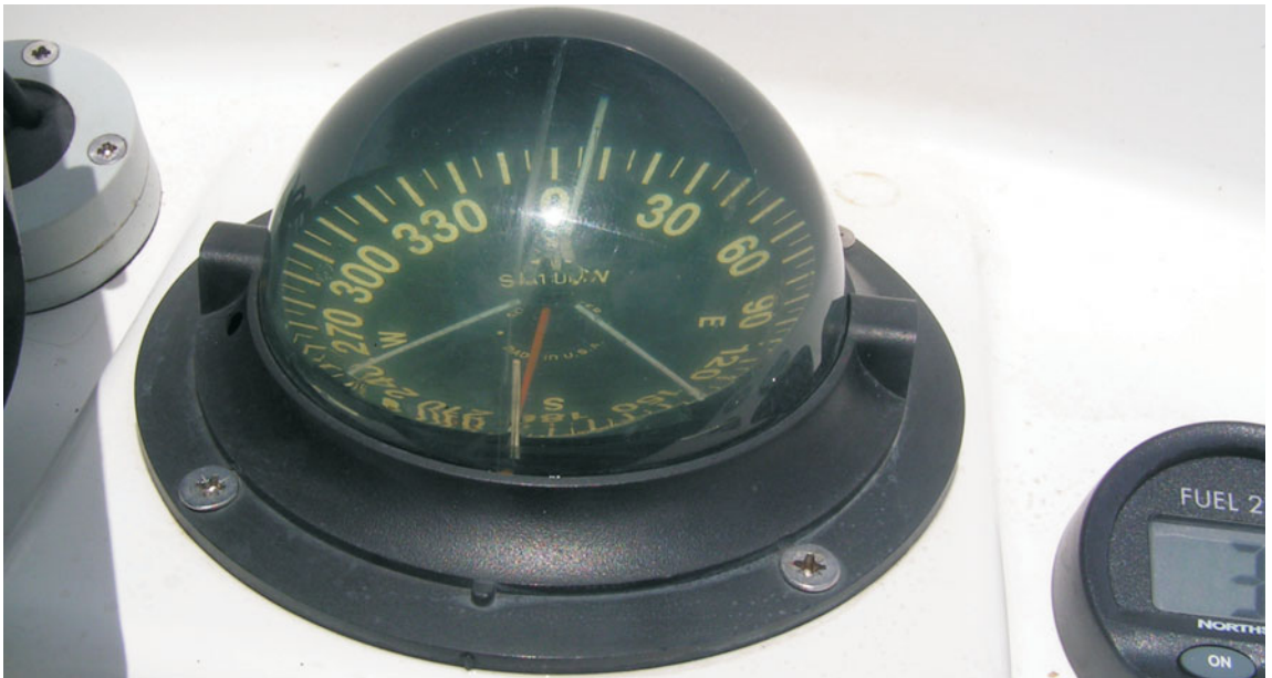
Fig 13b A flush-mounted steering compass on a fast sportsboat.
