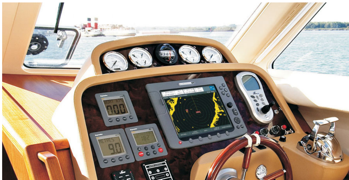
Fig 89 A flush-mounted multi-function display in radar mode, at the helm position of a new motor cruiser.
