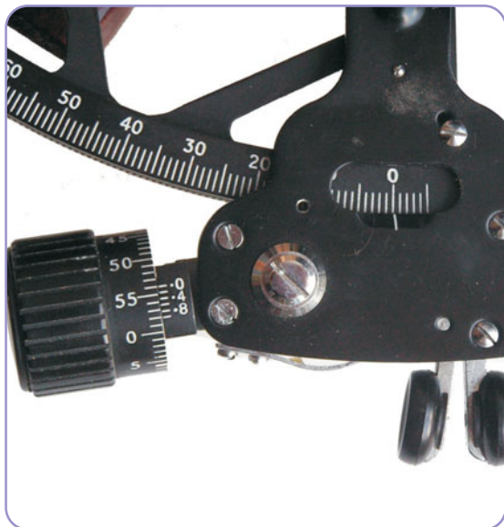
Fig 44 Before using a sextant, it must always be checked for index error – which makes the horizon look ‘broken’ when the sextant reads zero. Adjust the micrometer drum to make the horizon look straight, and read off the index error (see text).
