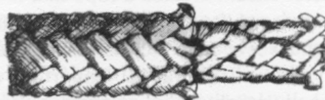
Double braid rope showing the braided sheath and braided core.
