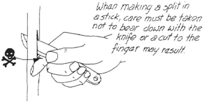
Using the knife as a shear.
