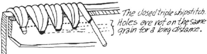
Detail of durable rim construction.
