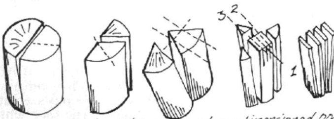
How to make rectangular-dimensioned boards.
