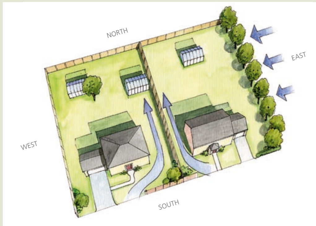
The ideal greenhouse location is well away from trees but protected from prevailing winds, usually by another structure, a fence or a wall.
