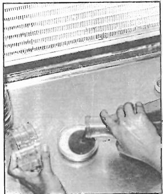
Figures 68-69. Pouring malt agar into sterile petri dishes in front of laminar flow hood.
