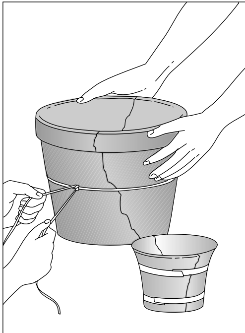
Figure 17-3: Using rope or tape can help you repair a broken pot.
