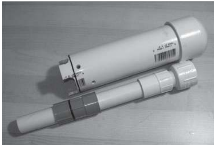
The large diameter at the top of an Affnan-style standpipe increases the range of flow rates that allow a bell siphon to function properly. This version of the Affnan-style standpipe uses parts commonly available in the United States.
