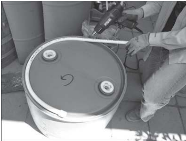
Bending PVC pipe to shape. The bent pipe will be used to prevent the open barrel from sagging.
