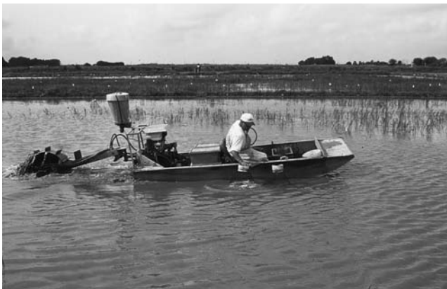
Figure 10. Hydraulic propulsion boats are commonly used to harvest crawfish in ponds. The broadcast distributor mounted on the rear was used for experimental feeding studies.
