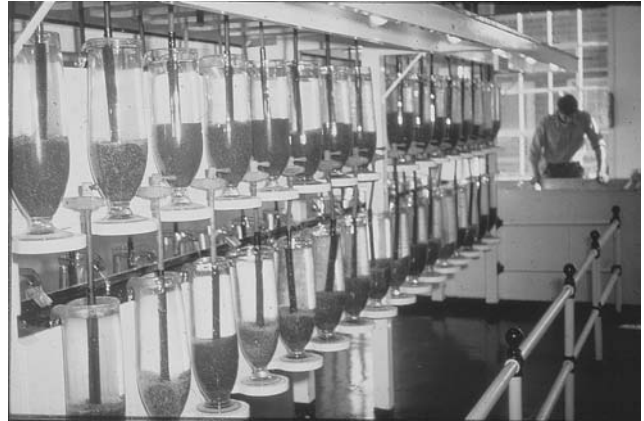
Figure 2. Large-scale, walleye incubation facility with many hatching jars. On hatch, the larvae swim to the top of the jar and go with the flow to a holding (catch) tank.
