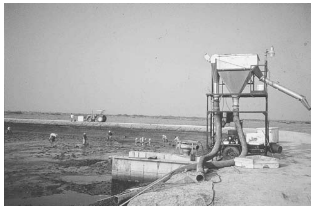
Figure 38. Automated harvester (Magic Valley Heliarc) at shrimp farm in Texas.
