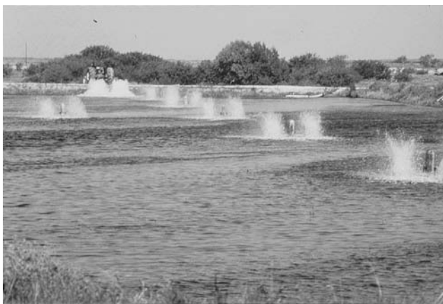
Figure 19. Paddlewheel aerators on 5-acre pond at Arroyo Aquaculture Association farm. (Photo by Louis Hamper.)
