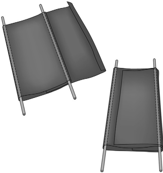
FIGURE 57-12 Improving a stretcher from two rigid poles and a blanket or tarp.
