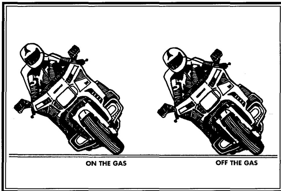
Rolling on the gas helps keep the bike up on the suspension, and that improves leanover clearance.
