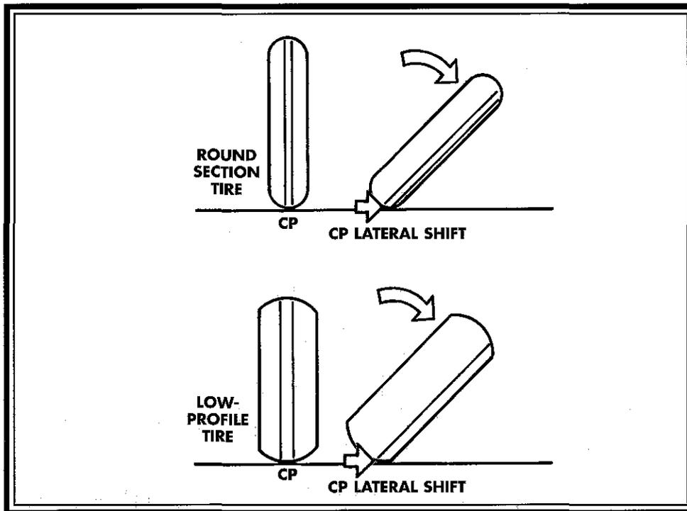
A low-profile tire experiences greater lateral shift of the CP than a round section tire when leaned over.
