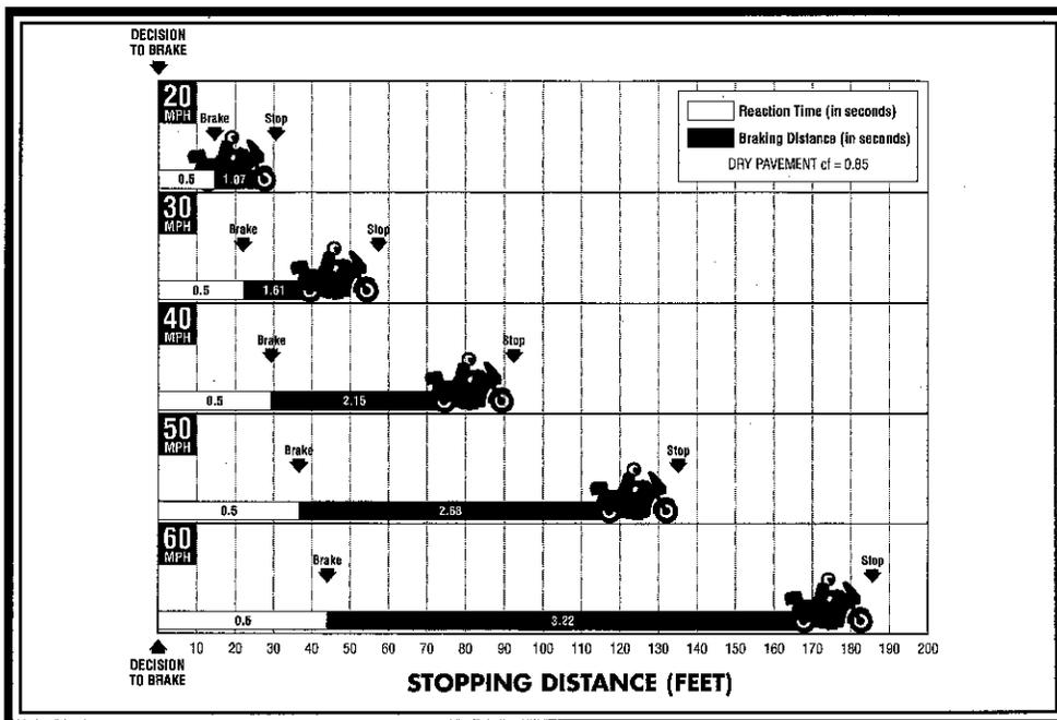
Including a half-second reaction time, a proficient rider can stop the typical bike going 40 mph in less than 100 feet.
