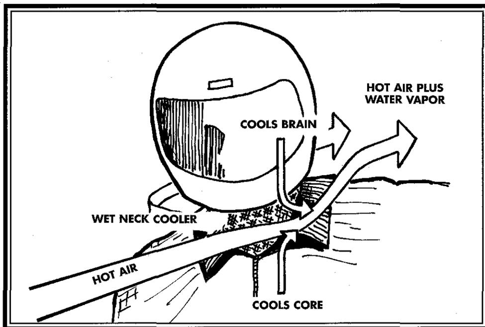
Water evaporating from a neck cooler absorbs heat from the neck and transfers it to the air, even if the air is hotter than the body.
