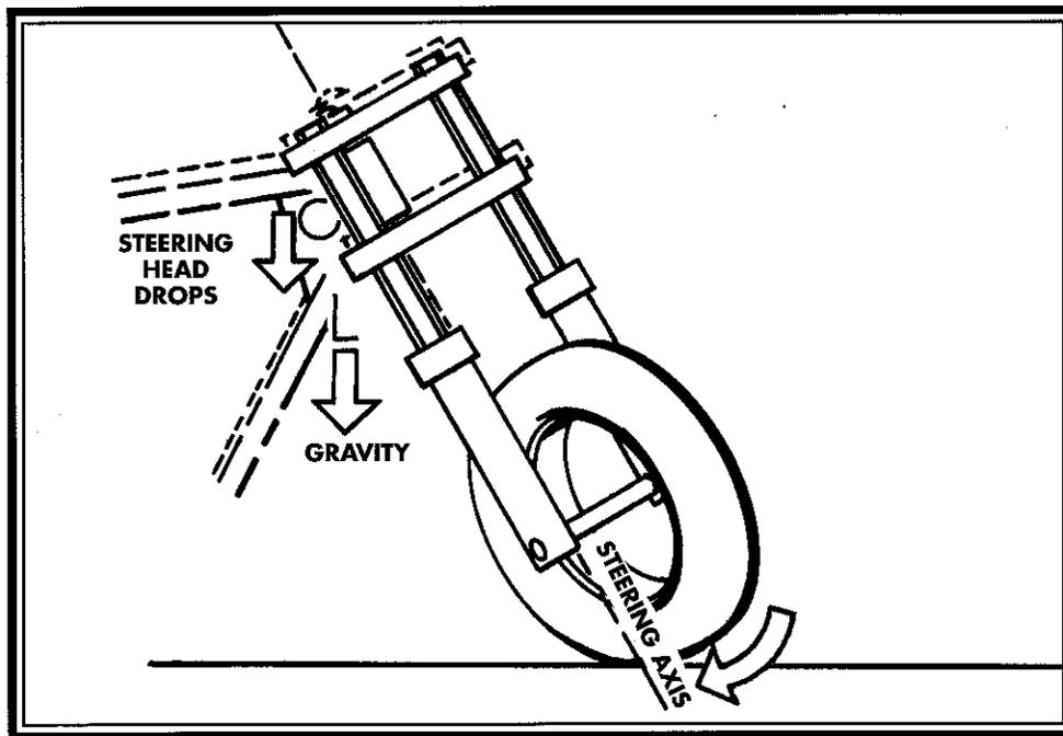
Because of rake, the steering head actually rises and falls when the front end is steered.
