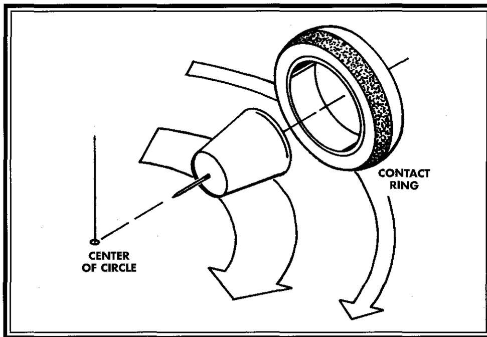
When the tire is leaned over, the contact ring forms a cone, similar to the shape of a foam coffee cup.
