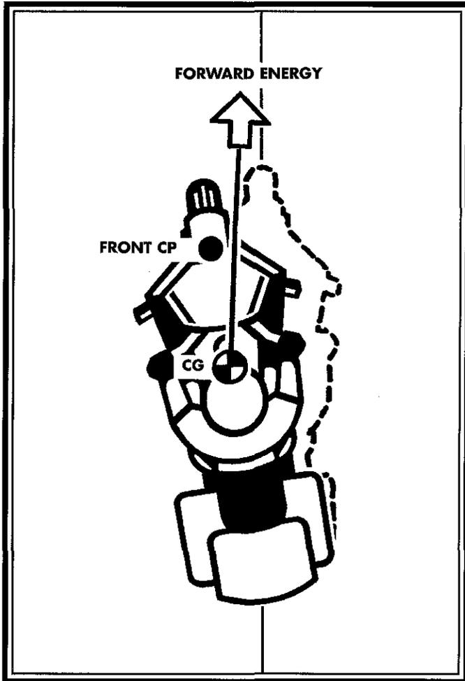
Even if the front wheel tracks off on a tangent, forward energy attempts to pull the bike back into a straight line again.
