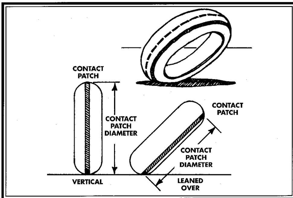
When the tire leans over, the contact ring moves toward the sidewall. You need to roll on the throttle just to maintain the same speed.
