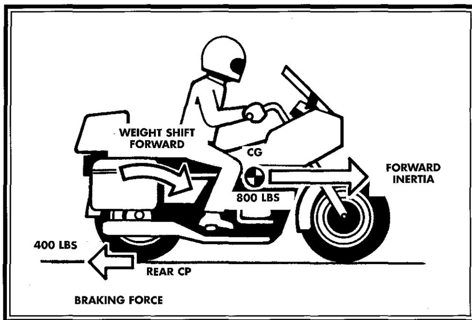
Braking force is proportional to the weight on the tire.
