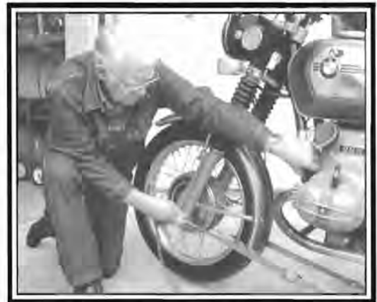
A tie-down strap keeps a centerstand or sidestand from retracting when you're working on the bike.
