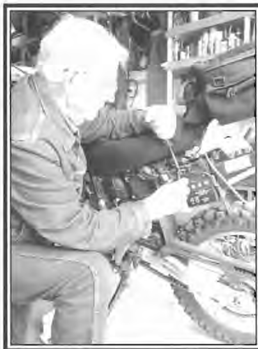
When you are connecting or disconnecting a battery, the hot tip is to disconnect the negative (ground) cable first when removing the battery; connect the negative cable last when installing.
