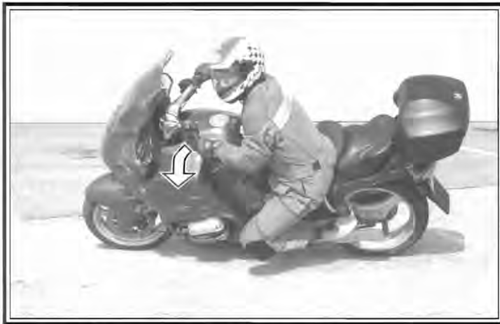
It's okay to think that you are pushing the bike over by pushing down on the grip.
