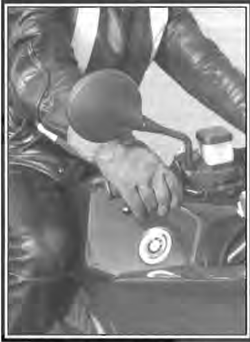
You should be able to squeeze firmly without the lever contacting the grip.
