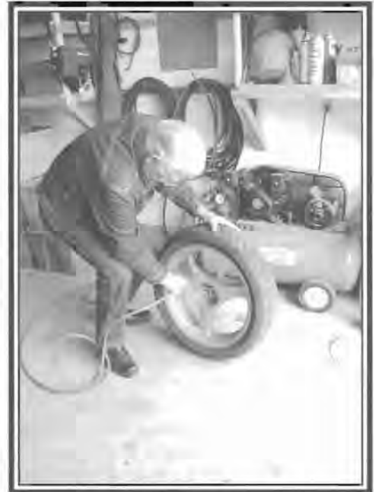
When popping the bead, hold the wheel upright, point the side of the wheel away from you, and don't exceed the recommended pressures.
