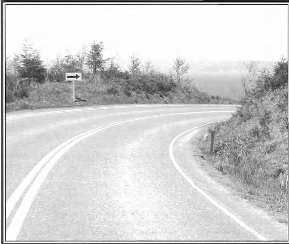
If you can see the opposite edge continuing around the turn, that's a good clue that the road is cambered to your advantage.
