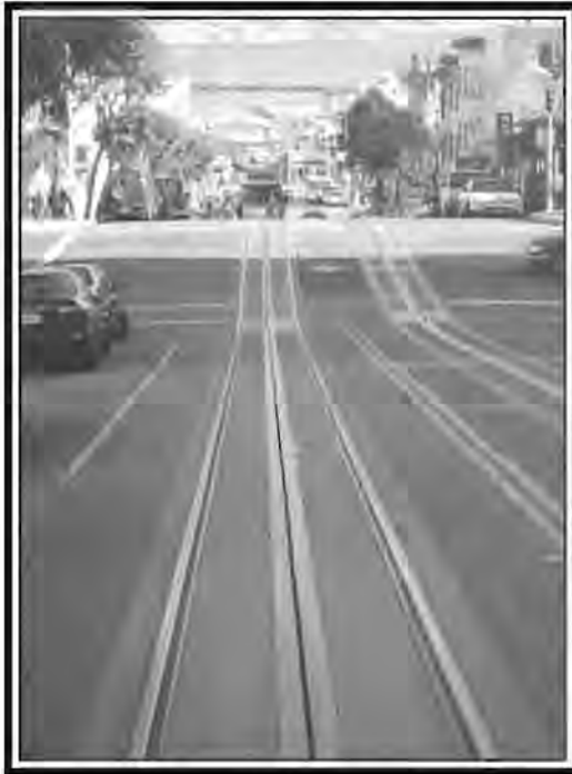
If you're sightseeing in San Francisco, pay close attention to those cable car tracks with the extra slot between the rails.
