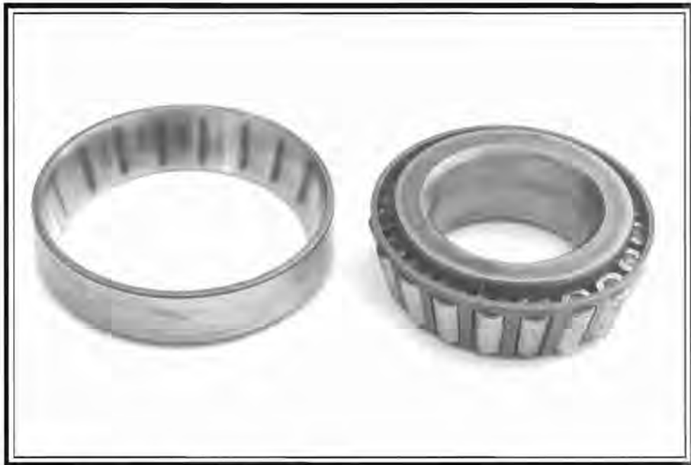
Notched steering head bearings result in vague steering.
