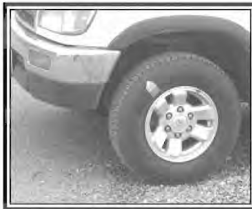
The top of the tire moves twice as fast as the car.
