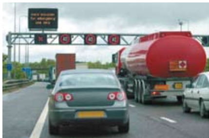
Rule 269 – Overhead gantry showing red cross over hard shoulder
