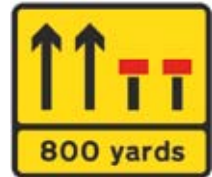
Temporary lane closure (the number and position of arrows and red bars may be varied according to lanes open and closed)
