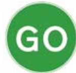
Manually operated temporary GO sign
