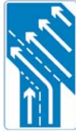
Traffic in right hand lane of slip road joining the main carriageway has priority over left hand lane
