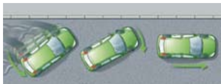
Rule 119 – Rear of the car skids to the right. Driver steers to the right
