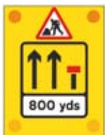
Signs used on the back of slow-moving or stationary vehicles warning of a lane closed ahead by a works vehicle. There are no cones on the road
