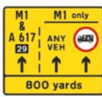
Lane restrictions at road works ahead
