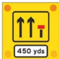
Signs used on the back of slow-moving or stationary vehicles warning of a lane closed ahead by a works vehicle. There are no cones on the road
