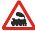
Level crossing without barrier or gate ahead
