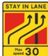
One lane crossover at contraflow road works
