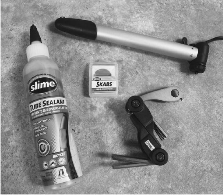
Sample bicycle repair kit with multi-wrench, patch kit, Slime Tire Sealant, and hand pump
