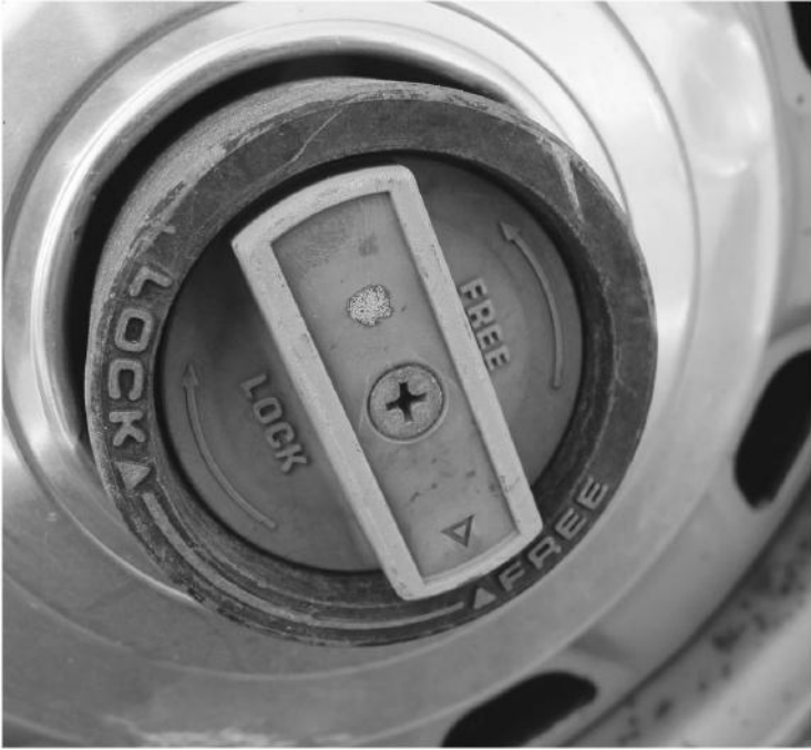
Manual locking hubs on front tires
