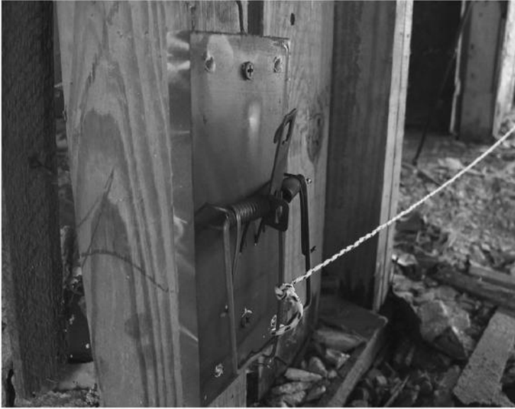
DIY rat trap perimeter alarm
