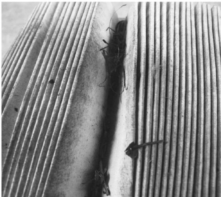
Clogged air filter
