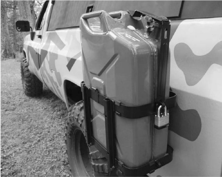
Five-gallon fuel jerry can mounted and secured with padlock to exterior of Creek's BOV
