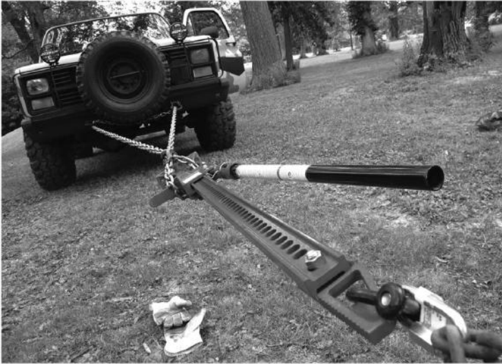
Hi-Lift Jack as a winching tool
