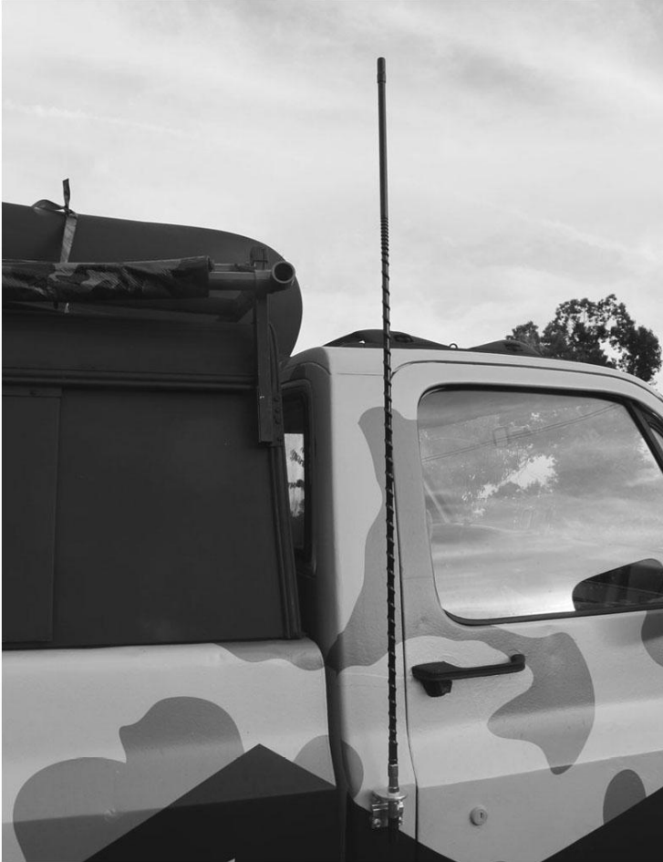
External CB antenna on Creek's BOV
