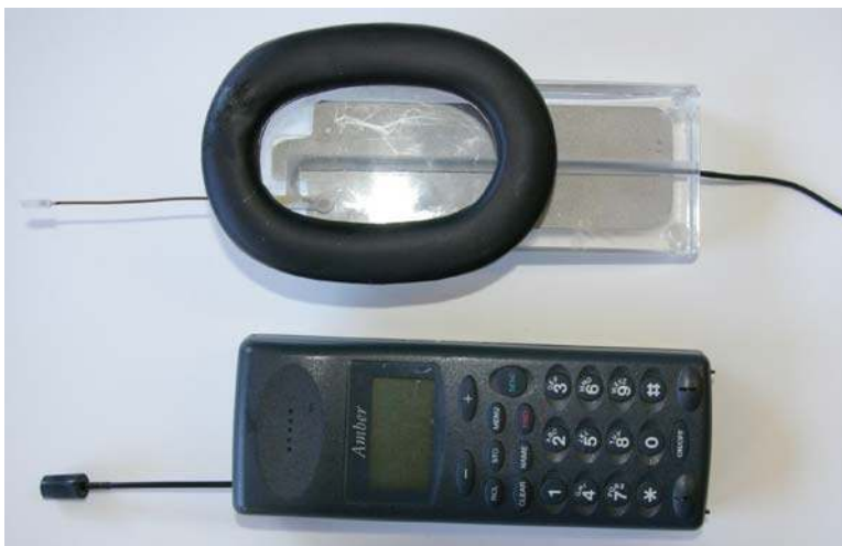
Figure 1. Model of an analogue 900 MHz using a sheet metal ground plane and simple quarter wave antenna pragmatically trimmed to resonance in proximity to the head. The soft ear muff locates the phone over the pinna. Since there is no battery or power module, heating from other than radiated power is minimal.
