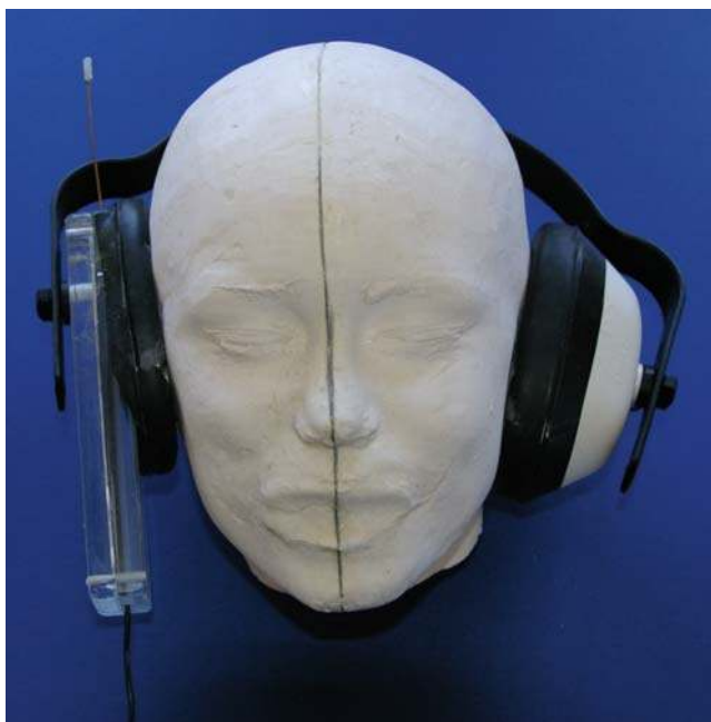
Figure 2. The simulated phone in position on a non-metallic ear defender. The plaster cast is that of a 10-year old used to model the acrylic shell for a realistic head phantom of a child (cast and shell produced by the mould room of the Oncology Centre, Bristol, UK).
