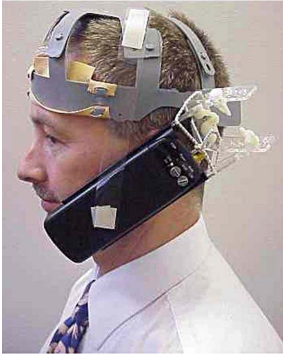
Figure 3. The MTHR setup used for a GSM phone simulation. In this case the phone is more controlled in position, and is a self contained unit transmitting GSM, or constant wave, or transmitting into an internal dummy load. This means that the total power consumption will be constant, although there may be slightly more power dissipated in the phone as a result of the power deposited in the load as opposed to that radiated in the active state (Photo courtesy of Phil Chadwick).
