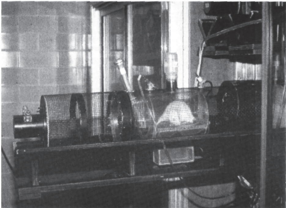
Wave guide system showing rats are unrestrained and thus their whole bodies are exposed to radiation, not just their heads. This design was rejected by Carlo's researchers as inadequate for cellular phone studies.
