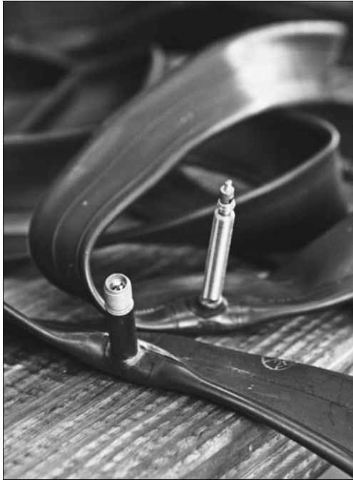
Figure 6-2: Tubes feature one of two types of valves: a Presta valve (left) or a Schrader valve (right).
