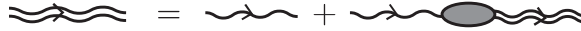
Figure 11.17 Phonon Green's function in the random phase approximation. The shaded bubble is the polarizability of interacting electrons. The single wavy line represents the bare (noninteracting) phonon Green's function, while the double wavy line represents the dressed (interacting) phonon Green's function.
