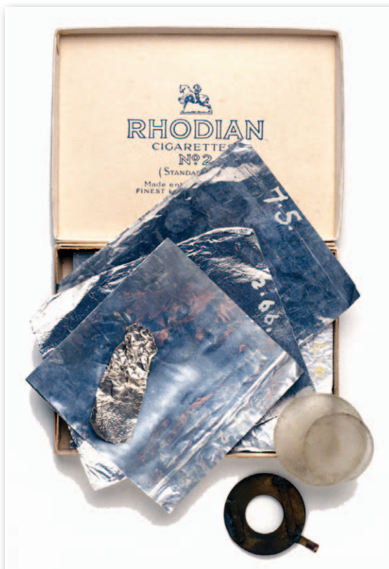
James Chadwick's toolbox held paraffin as well as aluminium and silver foils, which he used with his neutron detector. SSPL via Getty Images
