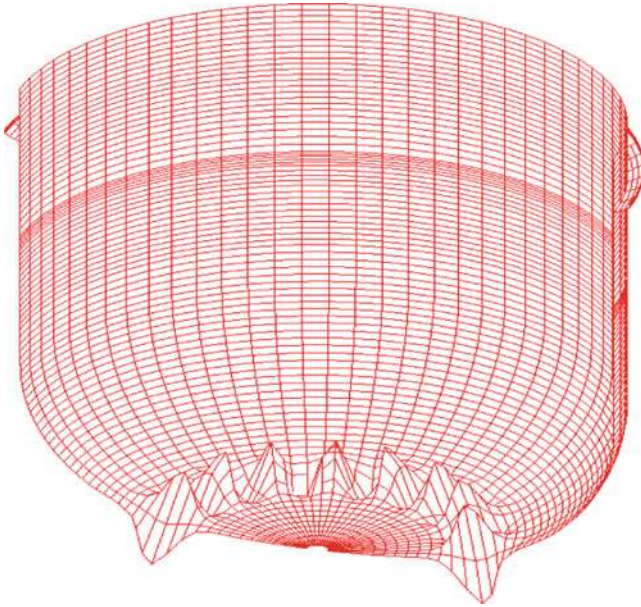
■ Figure 220 Buckled mode shape of safety vessel
