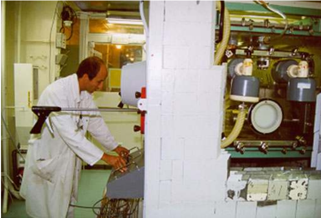
■ Figure 68 Shielded cell for handling active samples
