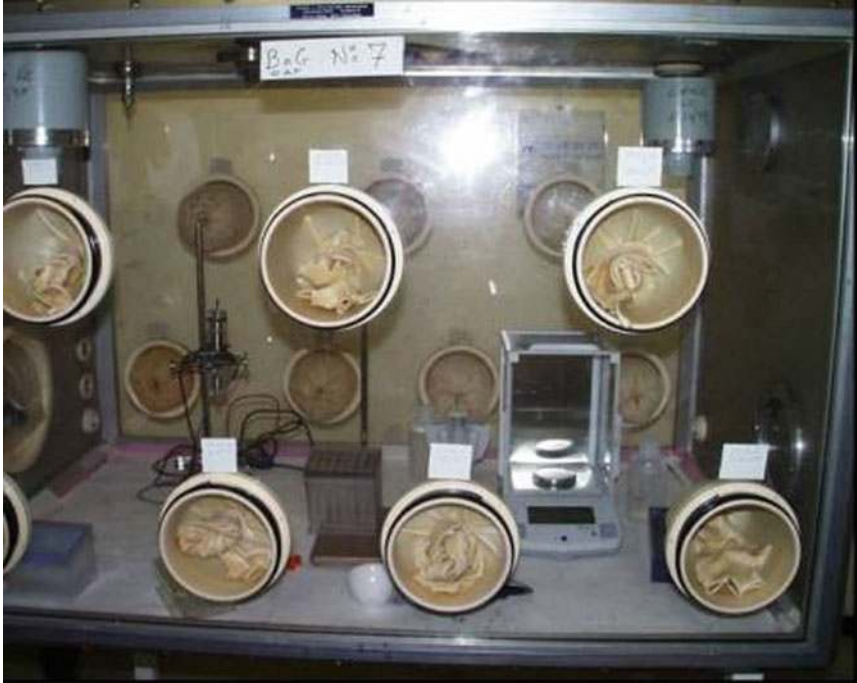
■ Figure 55 Glove box holding electrodepositions
