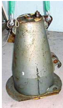
■ Figure 69 "Milk can" for transferring samples from the cell to the MINERVE reactor chimney
