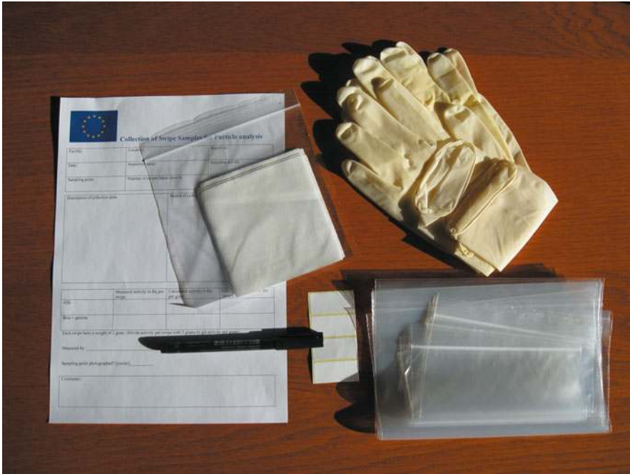
■ Figure 32 Sample kit for dust sampling using cotton swipes
