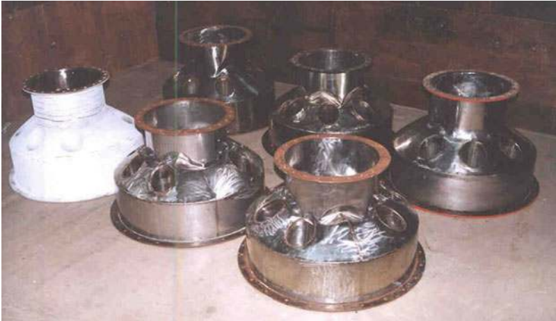
■ Figure 231 Buckled mode shapes of inner vessel models
