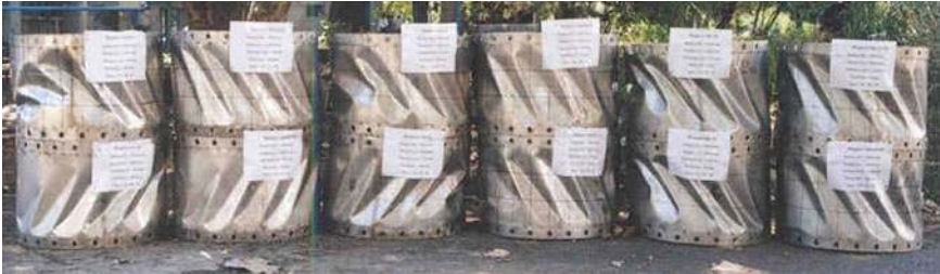
■ Figure 228 Buckled shells (1/18th model of main vessel) vessels under shear
