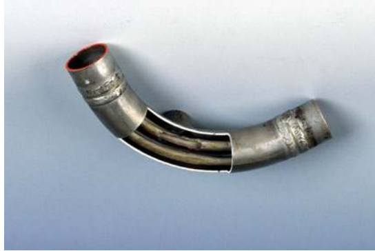
■ Figure 16 Hydrogen-meter based on Ni diffusion
