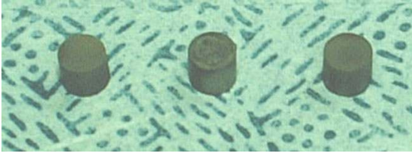
■ Figure 70 Example of fuel pellets for the OSMOSE program
