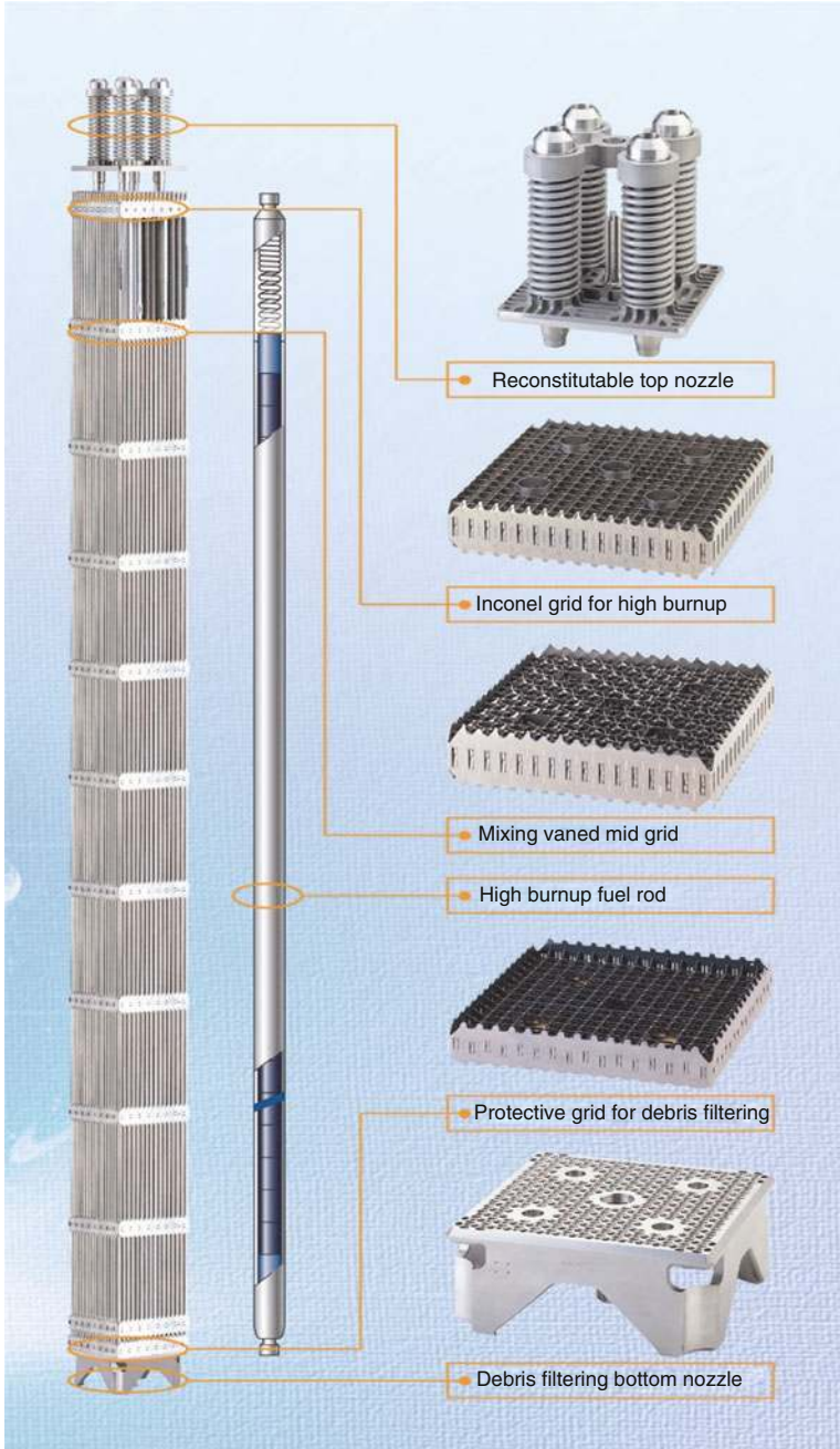
Figure 13 PLUS7 fuel assembly (Courtesy of Korea Nuclear Fuel Co., Ltd.)
