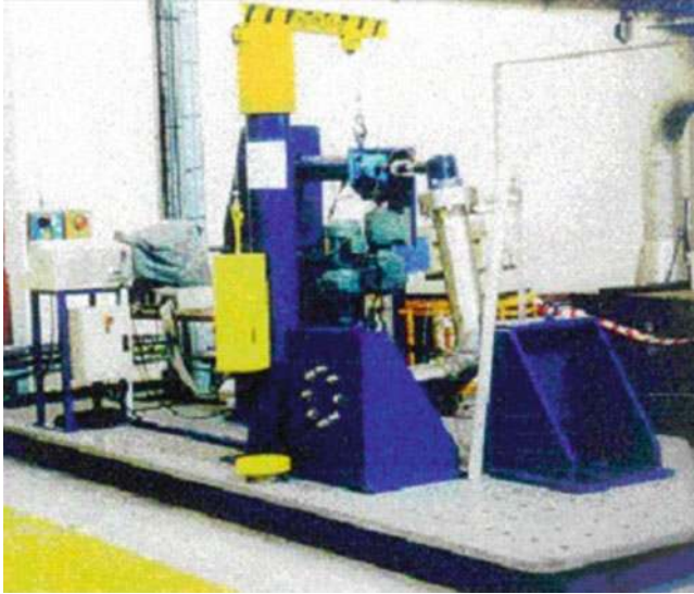
■ Figure 186 Actuator system for testing elbows
