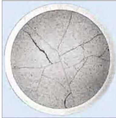
Figure 73 Radial macrograph of a spent fuel pellet
