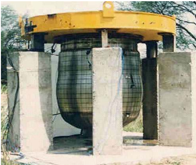
■ Figure 268 Deformed MV (1,200 MJ case)
