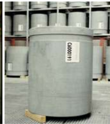
Technological waste enrobed in concrete
