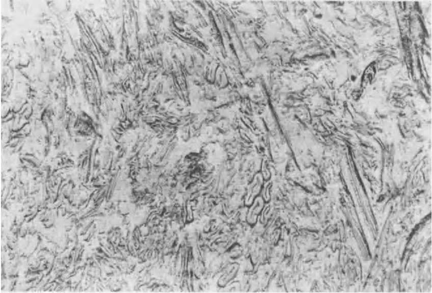
FIGURE 4.2. Wood flour mounted in black phenolic resin. Polished cross section, reflected light. The fibers are straight in lengthwise section, and some cross sections occur in groups. (1)
