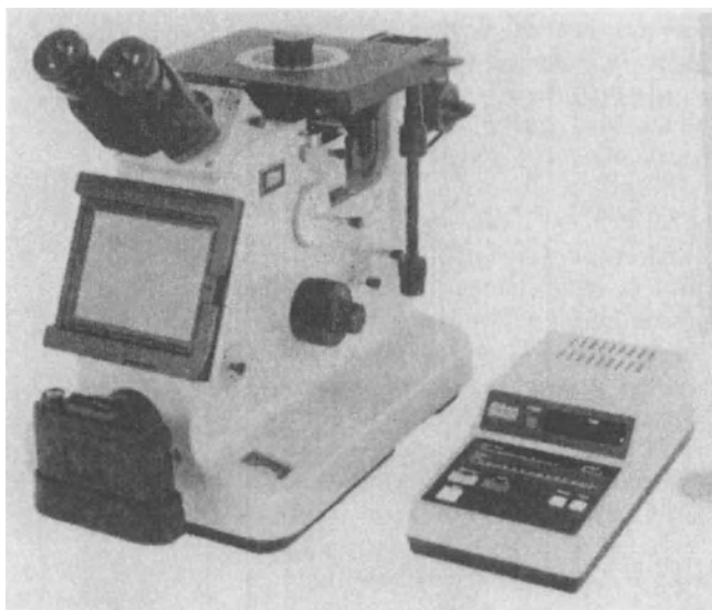
FIGURE 4.19. An inverted microscope arranged so that the briquetted specimen lies flat on its plane, polished face. Also fitted with large and small cameras. (16) Courtesy of Nikon.
