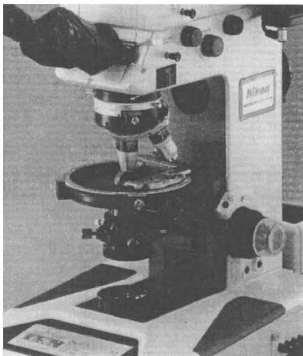
FIGURE 5.13. Nikon microscope precisely designed for microscopy by transmitted, polarized light, including photomicrography and television. (14) Courtesy of Nikon Instrument Group. (14)
