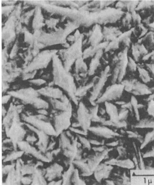
FIGURE 15.26. Pure gold wire before annealing. Compare with Figure 15.7 sample after annealing. (13) Courtesy of A. C. Reimschuessel.
