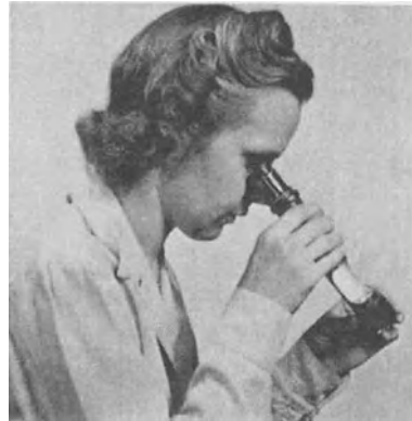
FIGURE 3.4. Hand compound microscope being used in micrometry by reflected light for opaque specimens. Courtesy of Helen Clapp.
