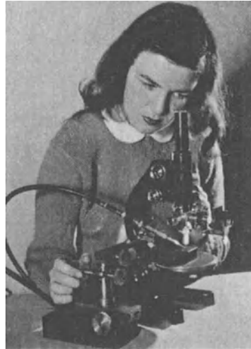
FIGURE 4.24. Dental drill and micromanipulator. The chuck of the dental drill is held in a special clamp attached to a micromanipulator. (1)
