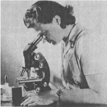
FIGURE 12.1. This biological microscope has a built-on, graduated mechanical stage. (2)
