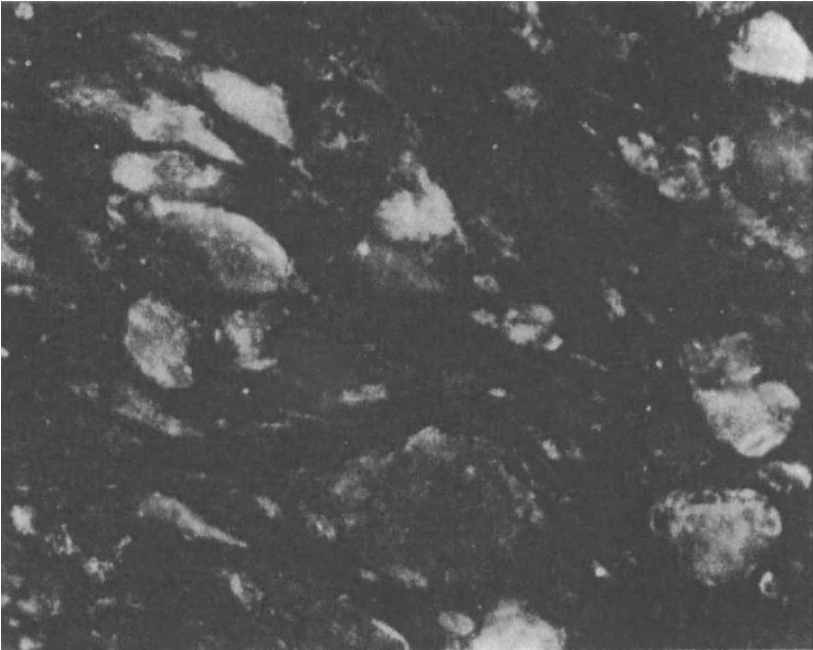
FIGURE 20.28. Elastic mixture or spread for one-step bonding of aluminum sheets. Continuous phase is phenolic varnish; particulate phase is an elastomer. (25)
