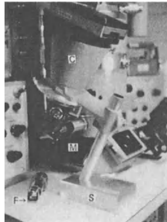
FIGURE 14.11. Polaroid® camera system attached to a TEM. A fluorescent crystal mirror assembly ( F ) is on table in foreground. (29)
