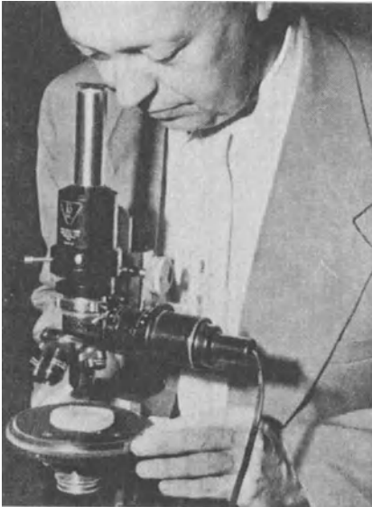
FIGURE 4.27. D. W. Davis using an all-purpose polarizing compound microscope, used in industrial microscopy with either reflected or transmitted illumination, bright field or dark field. Courtesy of American Cyanamid Co.
