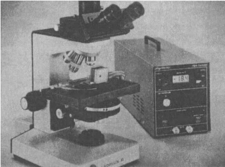
FIGURE 12.19. Thermal stage on a light microscope. Courtesy of Sensortek. (28)
