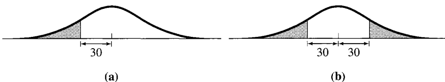
Figure 10.6. (a) The “one-tailed” probability for getting a result 30 or more below the mean. (b) The “two-tailed” probability for getting a result that differs from the mean by 30 or more in either direction. (Not to scale.)
