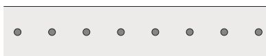
Fig. 6.6 A section through a multi-wire proportional chamber with thin aluminium Mylar windows acting as cathode and an array of fine anode wires, each providing gas amplification and a separate channel of electronic amplification (not shown).
