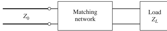
FIGURE 5.1 A lossless network matching an arbitrary load impedance to a transmission line.
