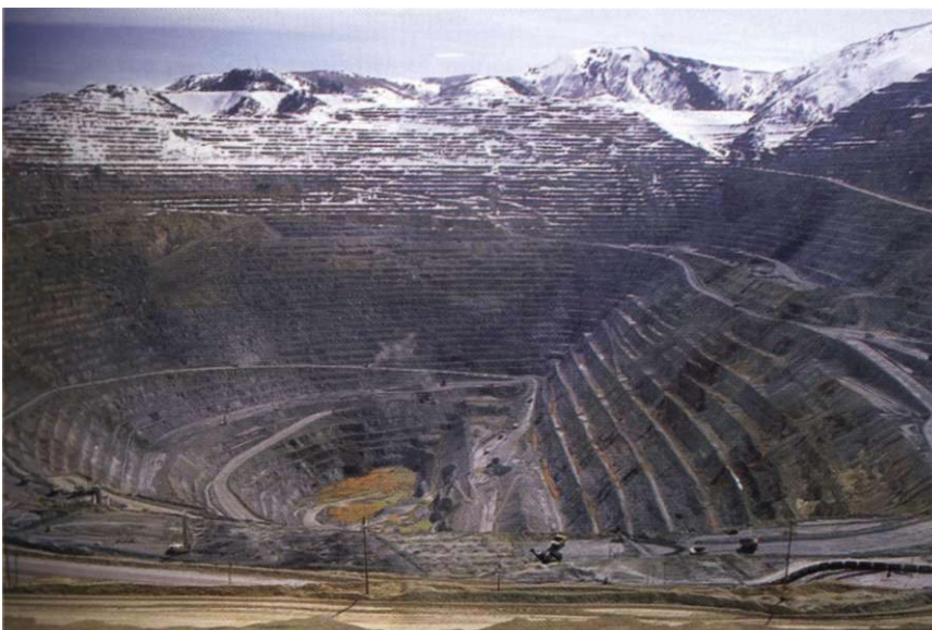
Figure 3.31 Kennecott Copper Mine, Utah, an open-pit mine. Open-pit mining is typical of the large-scale methods used to exploit widely disseminated ore deposits. [David R. Frazier/The Image Works.]
