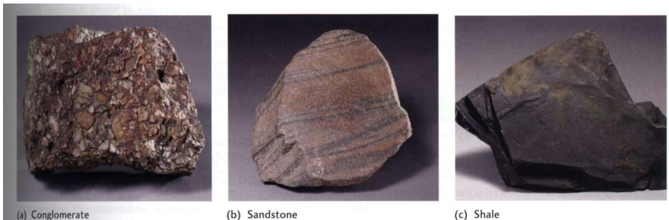
Figure 5.15 Clastic sedimentary rocks. [Conglomerate and sandstone: John Grotzinger/Ramón Rivera-Moret/MIT. Shale: John Grotzinger/Ramón Rivera-Moret/Harvard Mineralogical Museum.]
