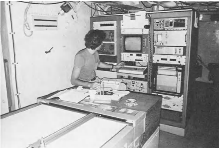
Figure 5. Survey Data Center on R/V PROSPECTOR. Data Recorder (left), Integrated Navigation System (center), Environmental Instruments, wave height analyzer and expandable STD (salinity-temperature-depth) recorder (right). Navigation plotter is in foreground.
