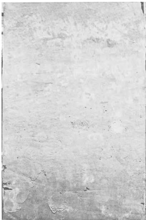
Figure 7. A box core of sediment. Material in cores are analyzed to provide information on nodule-sediment interface relationships, geotechnical properties, sediment texture, benthic biota and microfossils.
