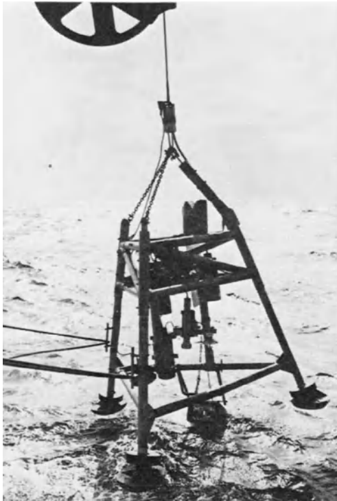
Figure 3. The deep-towed platform instrumented with television and still-cameras in the act of deployment from the R/V PROSPECTOR.
