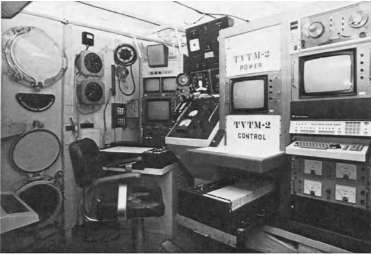
Figure 4. Survey Control Center on the R/V PROSPECTOR. Instrumentation displayed consists of a main winch control, TV screen, tape recorder, Integrated Navigation System, depth recorder, gyro compass.
