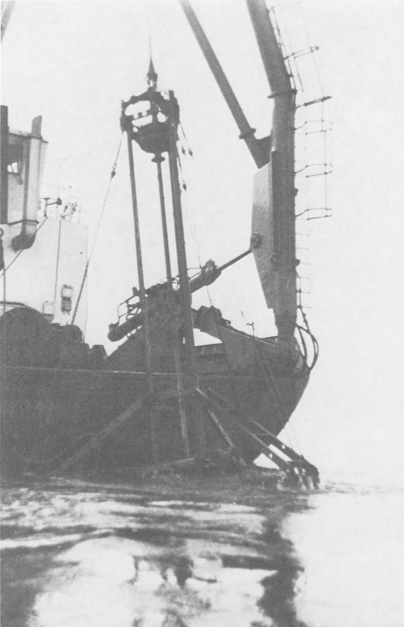
Figure 3. The BGS electric vibracorer being deployed from the stern of a support vessel by pivoting on the tension chains from a horizontal position on deck to a vertical attitude for lowering and operation.
